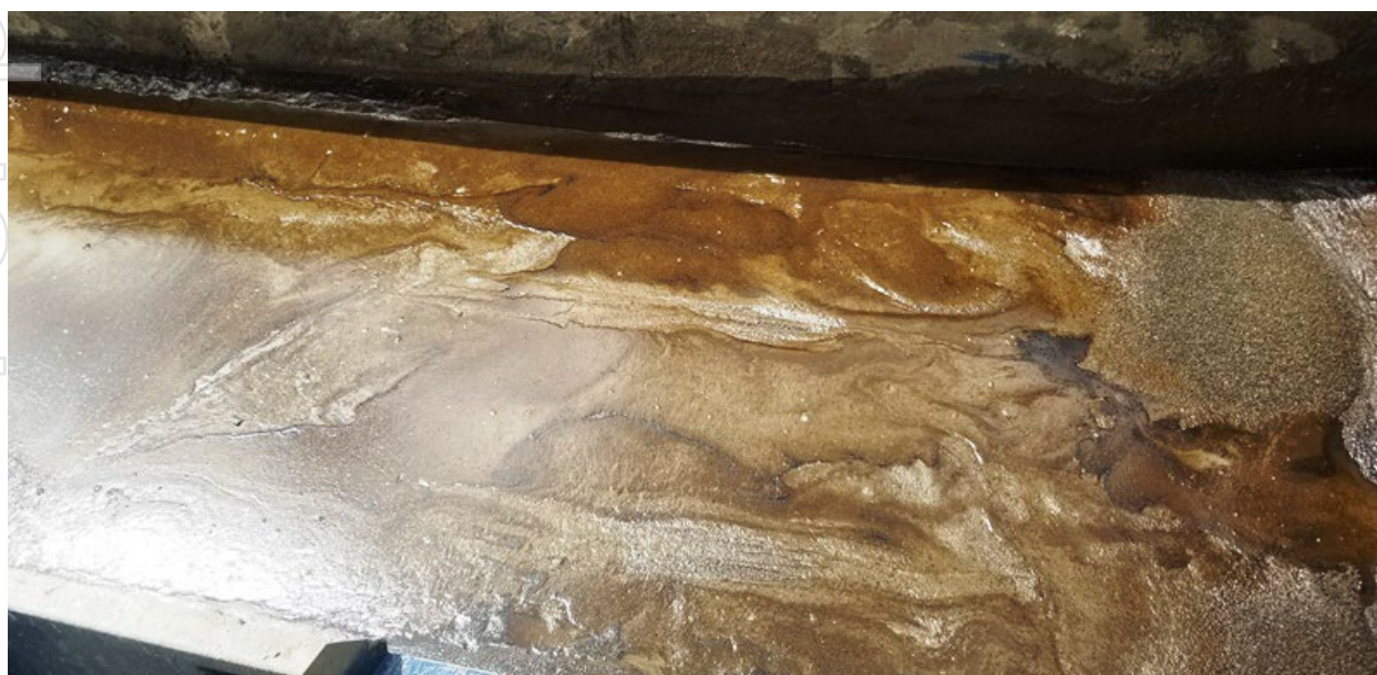
Figure 1 - Significant volumes of oil on the shakers at intercept of "N" structure
