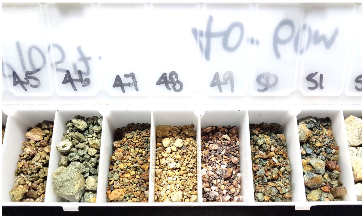
Figure 4: Quartz and hematite (±goethite) veining between 44m-49m including 1m @ 64.2 g/t Au between 48m-49m from RC21KP1057.
