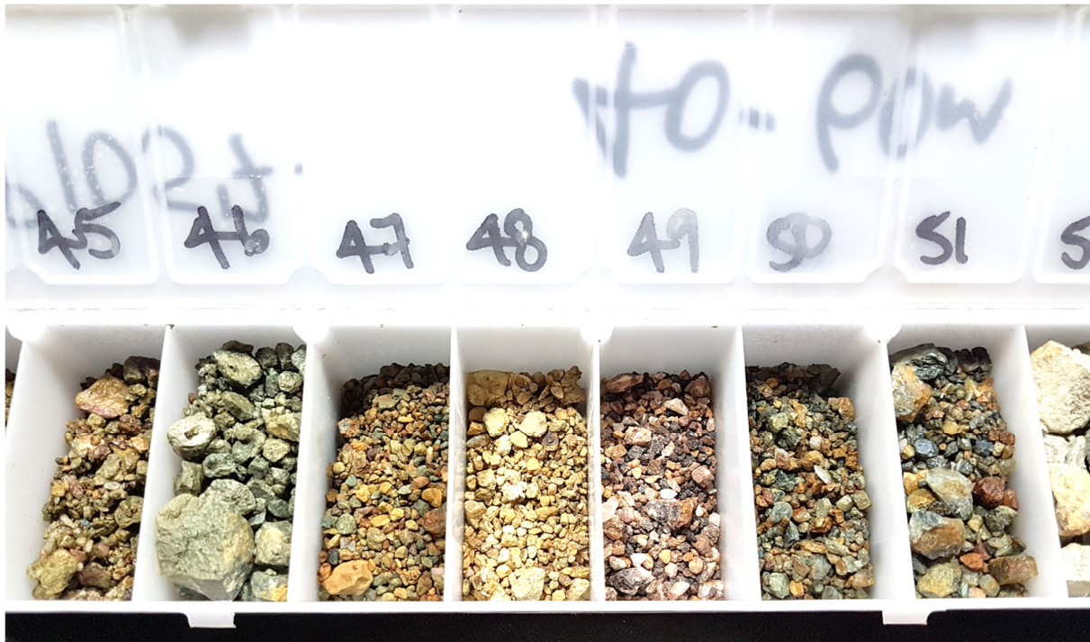
Figure 4: Quartz and hematite (±goethite) veining between 44m-49m including 1m @ 64.2 g/t Au between 48m-49m from RC21KP1057.
