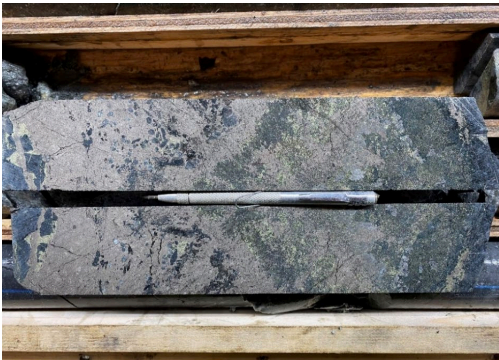
Figure 13. Core from drill hole JWD21-01 showing Cu-Ni-Co sulfarsenide mineralisation
