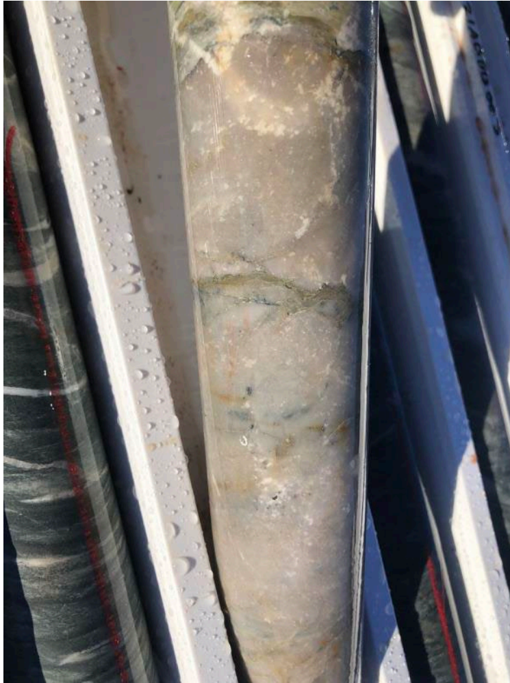
Figure 2 – 21ABDD003 (242.5-243m) showing silica flooding, carbonate altered interval with accessory pyrite, indicative of gold mineralisation.
