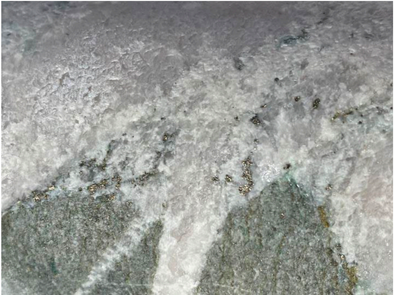
Figure 3 – 21ABDD001 (156.7-157.2m) close up of silica-carbonate alteration with associated 0.5-1% disseminated arsenopyrite-pyrite-chalcopyrite sulphide assemblage.
