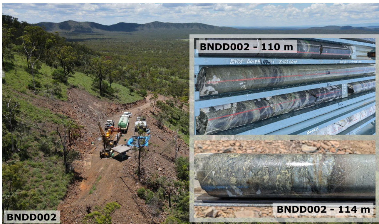
Figure 9. Isens drill rig set up on the pad drilling NW with examples of mineralised lodes intersected downhole.
