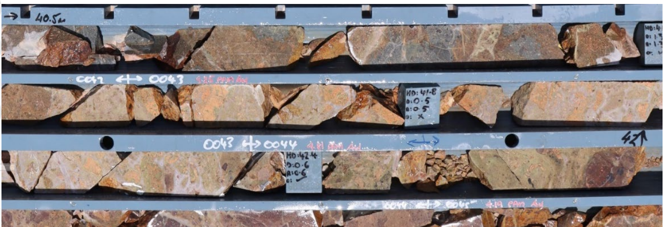
Figure 15. Brecciated volcaniclastic with colloform quartz infill associated with gold mineralisation in PCDD001 (interval 40.5 m to 43 m).
