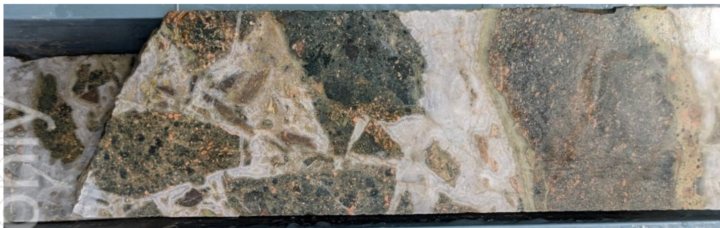
Figure 16. Close up of colloform quartz infill in PCDD001.
