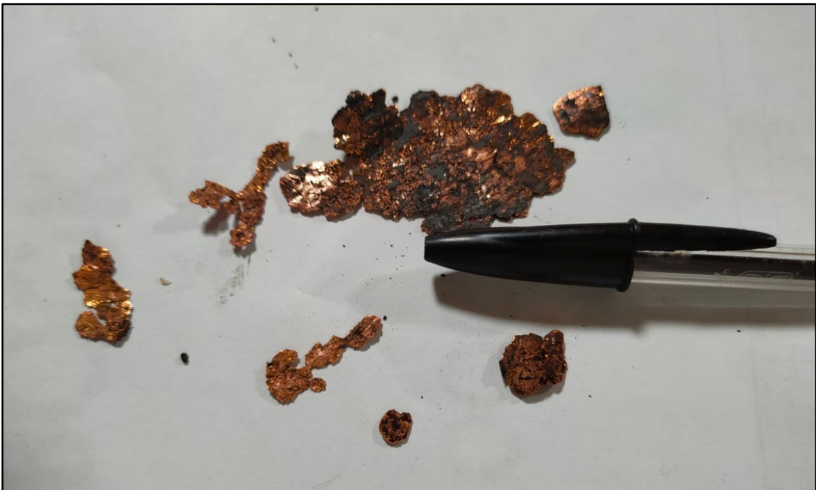
Image 6 | Native copper recovered from carbonaceous shale 21MDMT03, 114.6m
