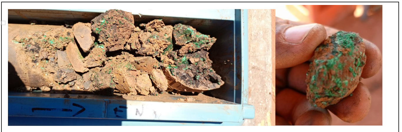
Image 9 | Malachite and chrysocolla mineralisation 87.2m 21MDMT01
