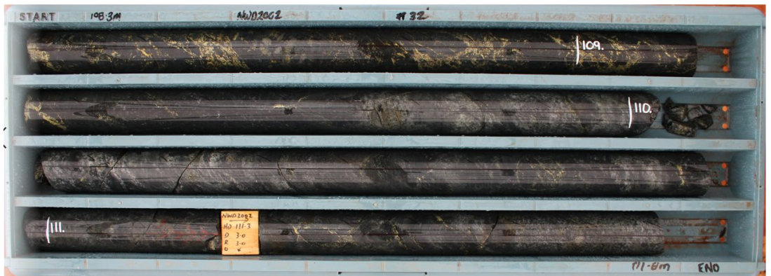
Image 12 | NWD2002: 107m to 109m; 2m @ 6.2% Cu, 0.5 g/t Au and 14.0 g/t Ag
