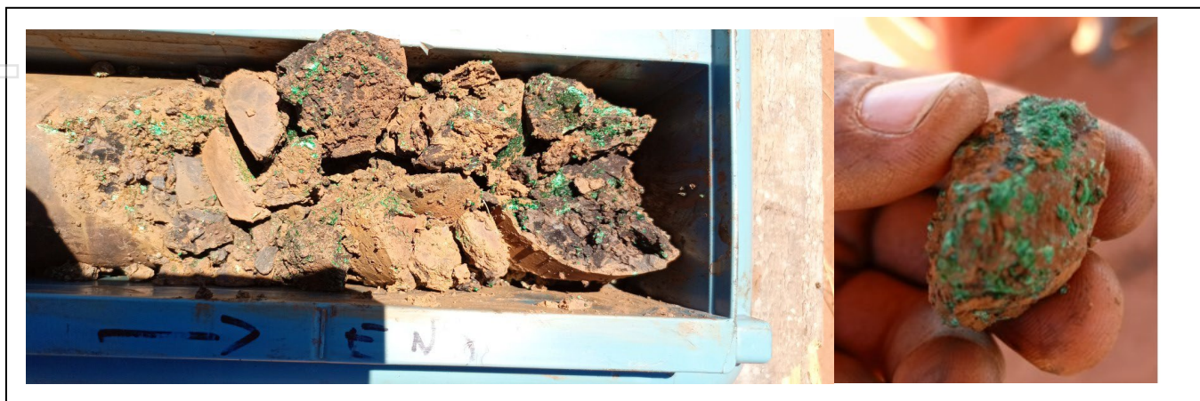
Image 9 | Malachite and chrysocolla mineralisation 87.2m 21MDMT01
