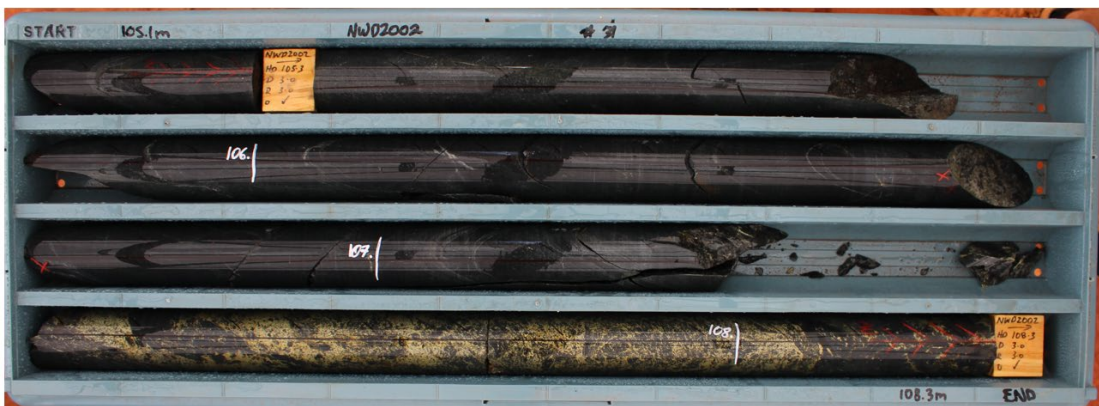
Image 11 / NWD2002: 64m to 66m; 2.0m @ 1.0% Cu, 0.2 g/t Au and 2.0 g/t Ag
