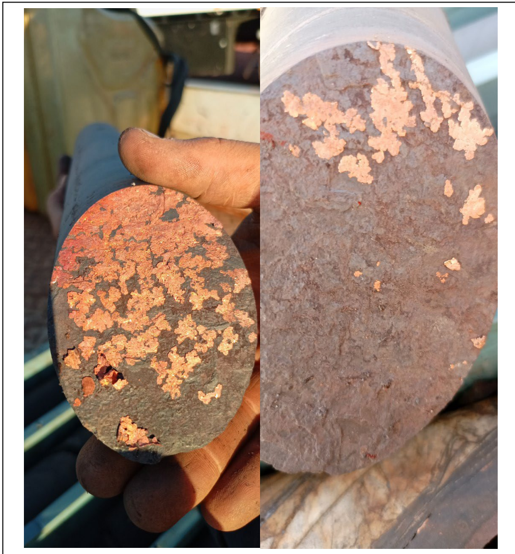
Image 8 | Native copper in carbonaceous shale 21MDMT03, 115.6m and 117.8m
