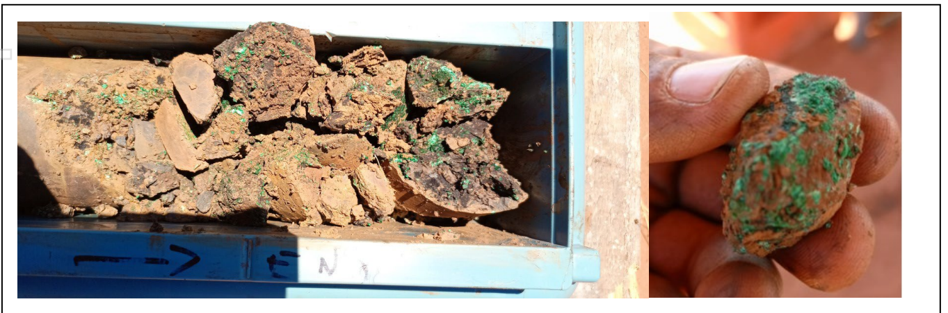
Image 9 | Malachite and chrysocolla mineralisation 87.2m 21MDMT01
