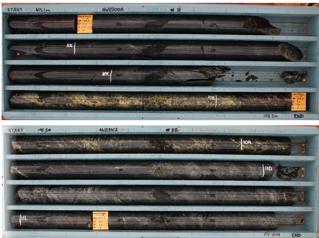
Image 12 / NWD2002: 107m to 109m; 2m @ 6.2% Cu, 0.5 g/t Au and 14.0 g/t Ag
