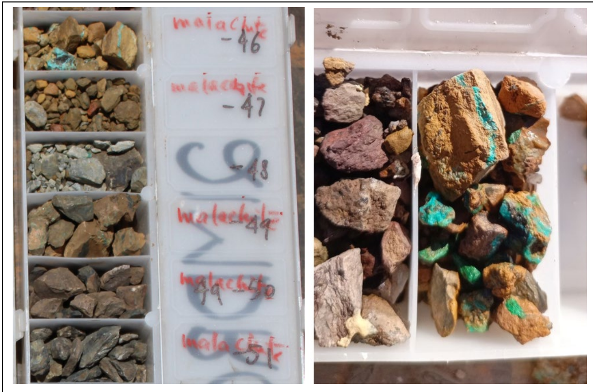
Image 4 | Malachite and Chrysocolla 46-51m 21MDRC016
