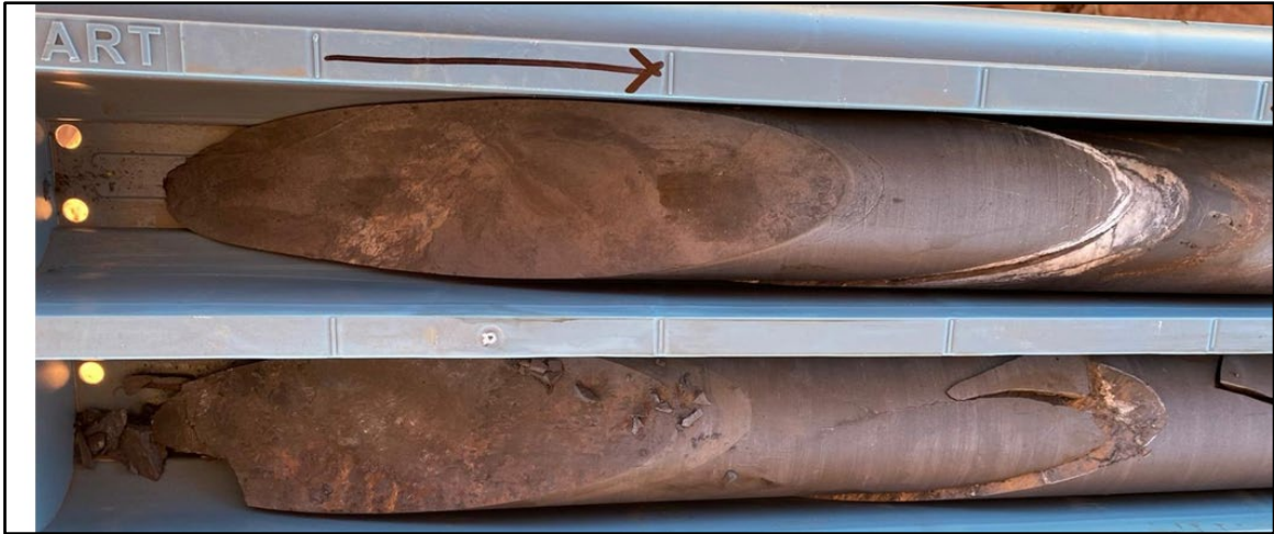
Image 10 | Native copper mineralisation 90.0m 21MDMT01
