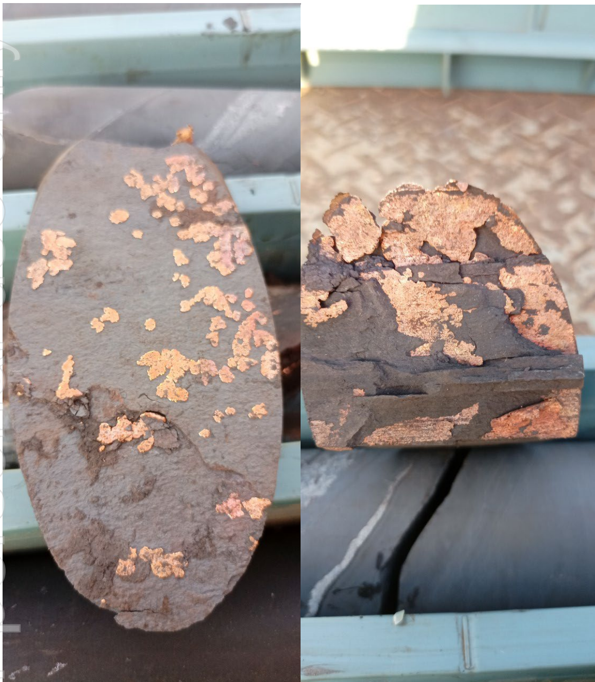
Image 7 | Native copper in carbonaceous shale 21MDMT03, 112.5m and 113.2m
