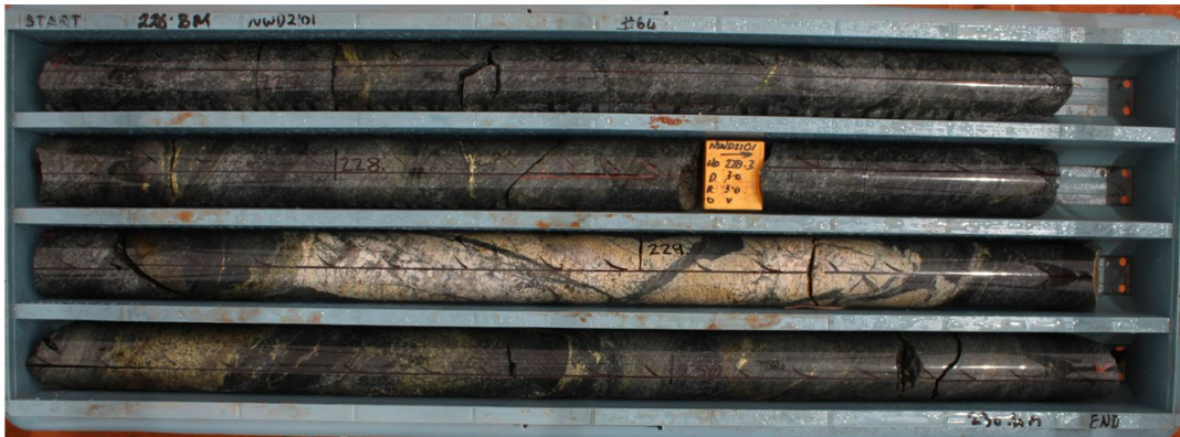
Image 13 | NWD2101: 222m to 224m; 2m @ 3.9% Cu, 0.8 g/t Au and 6.1 g/t Ag
