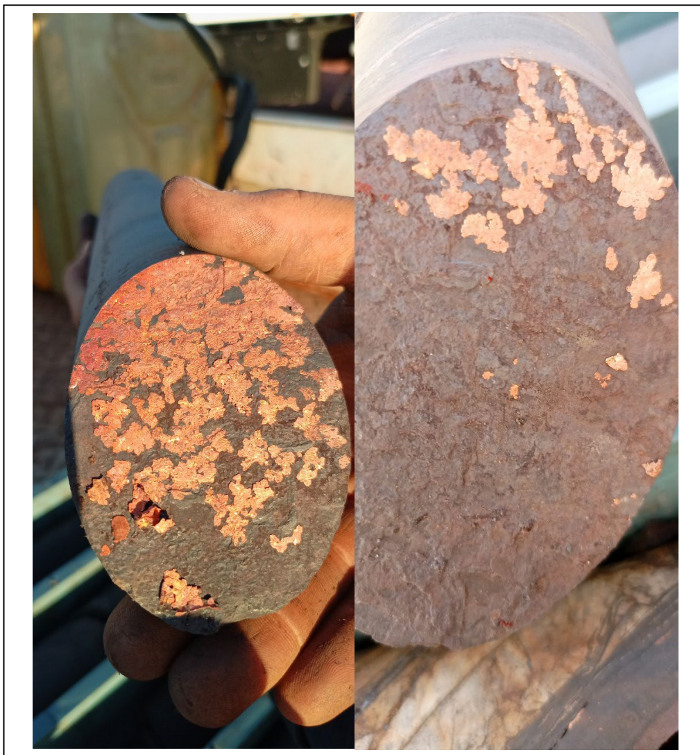
Image 8 | Native copper in carbonaceous shale 21MDMT03, 115.6m and 117.8m
