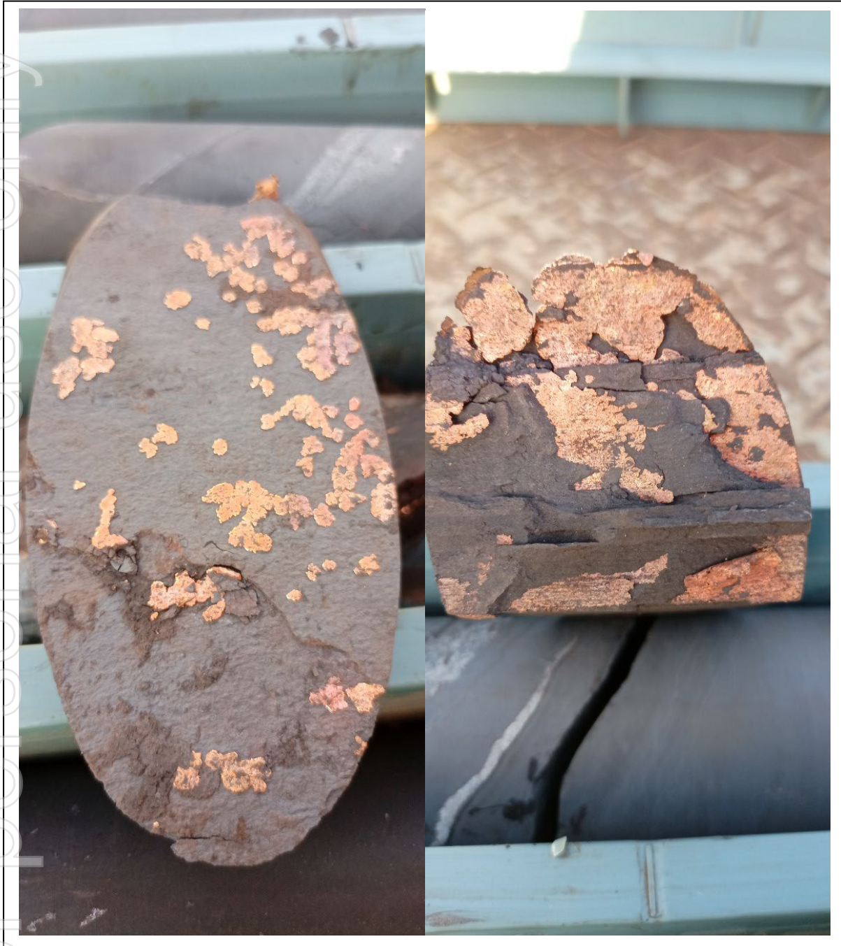
Image 7 | Native copper in carbonaceous shale 21MDMT03, 112.5m and 113.2m
