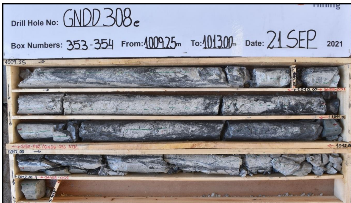
Photo 5 - Showing new mineralised zone from 1009 metres at the end of GNDD-308e
