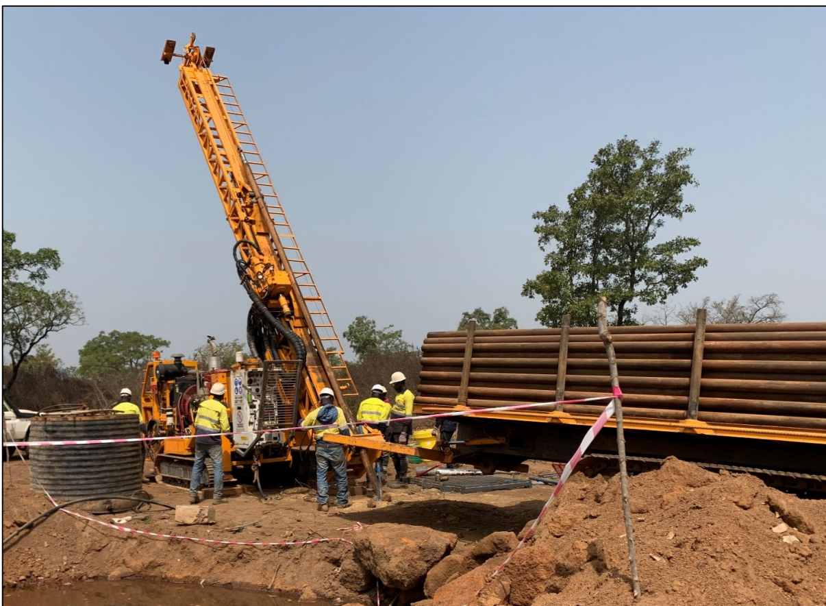
Figure 8: Diamond drill rig (DD) drilling at Tchaga
