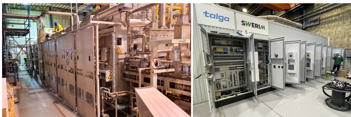
Figure 1 Part of Talga's Electric Vehicle Anode plant in Sweden; coating kiln (L) and electrical controls (R).
