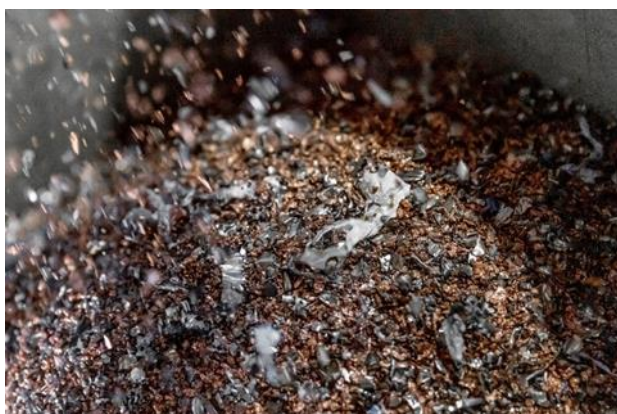
Figure 5 – Recovered Copper and Aluminium foil
