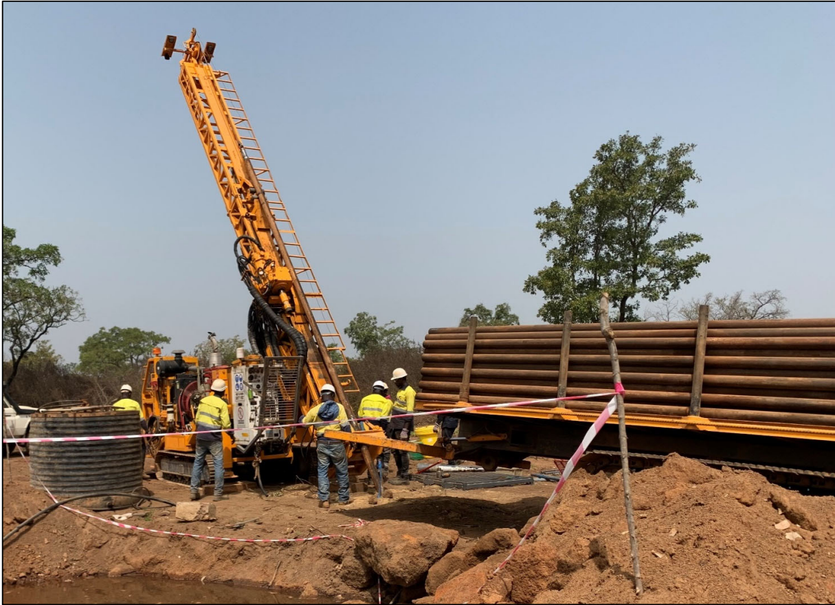
Figure 8: Diamond drill rig (DD) drilling at Tchaga
