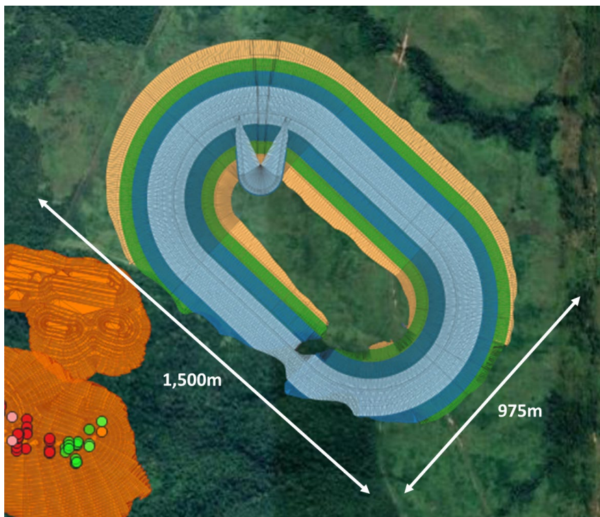
Figure 6: Tailings Storage Facility Design
