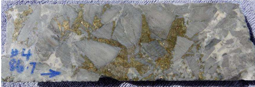
Fig 10 HQ Core photo hole 21CAEDD004, section 86.6m to 86.8 m, close up infill of chalcopyrite, pyrite in clast supported hornfels breccia. Primary zone 86m-87 assays 1m @ 2.58% Cu, 0.2 g/t Au, 78 g/t Ag (2 oz/t Ag) .
