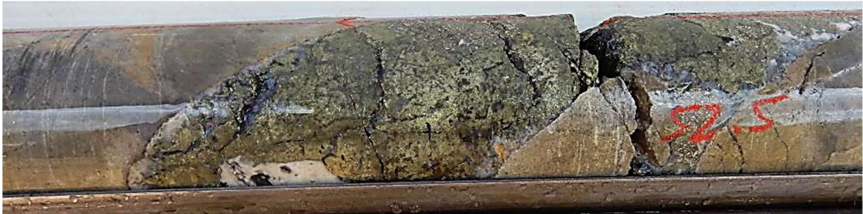
Fig 7 HQ Core photo hole 21CAEDD004, 52.5m. chalcopryite rich infill in clast supported hornfels breccia. Primary zone 52m-53m assays 1m @ 2.7% Cu, 7.9 g/t Au, 50 g/t Ag. (approx. 1.5 oz/t Ag)..
