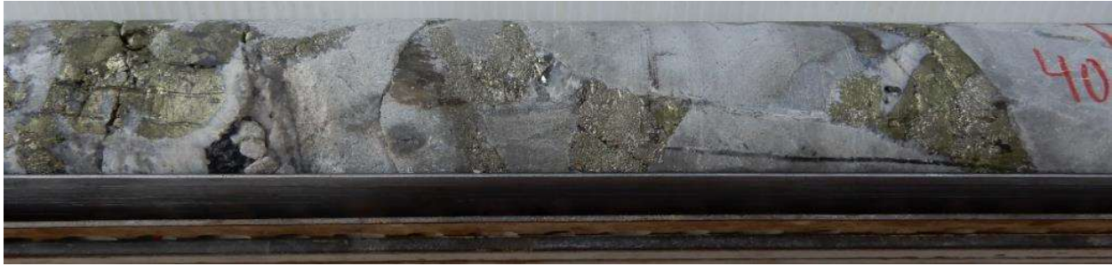
Fig 6 HQ Core photo hole 21CAEDD004, interval 40m to 40.2m. Pyrite and chalcopryite + quartz-carbonate infill in clast supported hornfels breccia. Primary zone 40m-41m assays 1m @ 2.62% Cu, 1.36 g/t Au, 46 g/t Ag. . (approx. 1.5 oz/t Ag).
