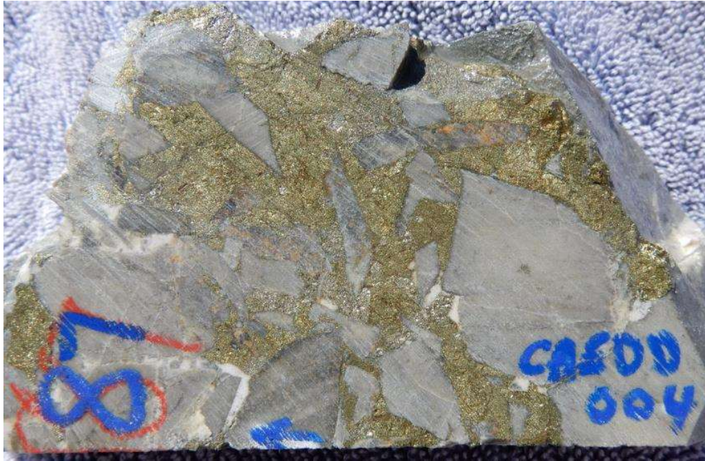
Fig 12 HQ Core photo hole 21CAEDD004, at 87m, infill of chalcopyrite, pyrite in clast supported hornfels breccia. 87m-88 assays, 1m @ 1.99% Cu, 0.14 g/t Au, 39 g/t Ag (1oz/t Ag).
