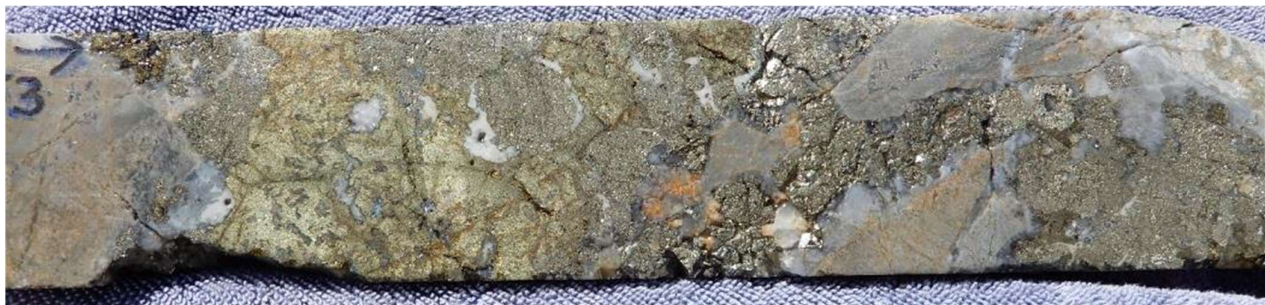
Fig 9 HQ Core photo hole 21CAEDD004, 53 to 53.5m-. close up infill of chalcopryite (golden), pyrite (brassy), carbonate (white) quartz (glassy) in clast supported hornfels breccia.
