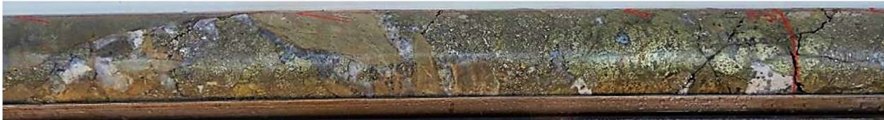
Fig 8 HQ Core photo hole 21CAEDD004, 53 to 53.5m-. infill of chalcopryite (golden), pyrite (brassy), carbonate (white) quartz (glassy) in clast supported hornfels breccia. Primary zone 53m-54m assays 1m @ 5.35% Cu, 5.71g/t Au, 88 g/t Ag. (approx. 3 oz/t Ag).
