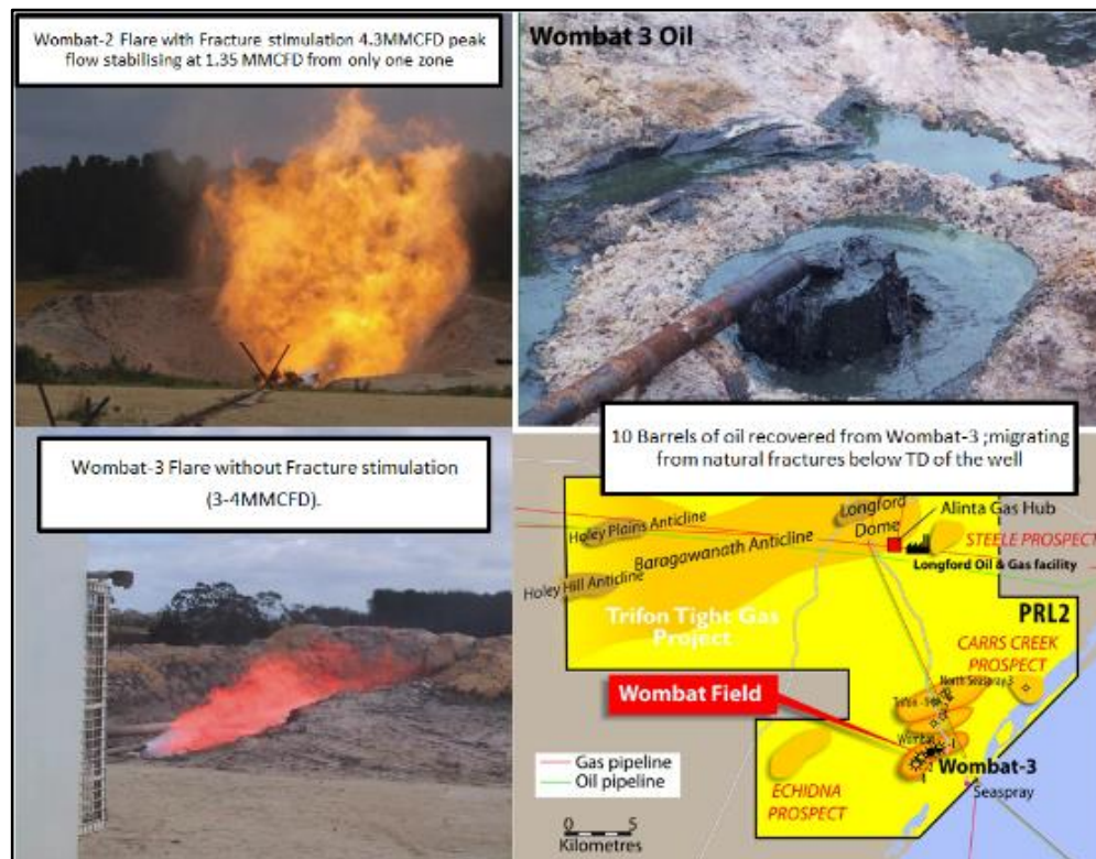
Figure 2-10: Wombat field example gas and oil flows obtained during testing
