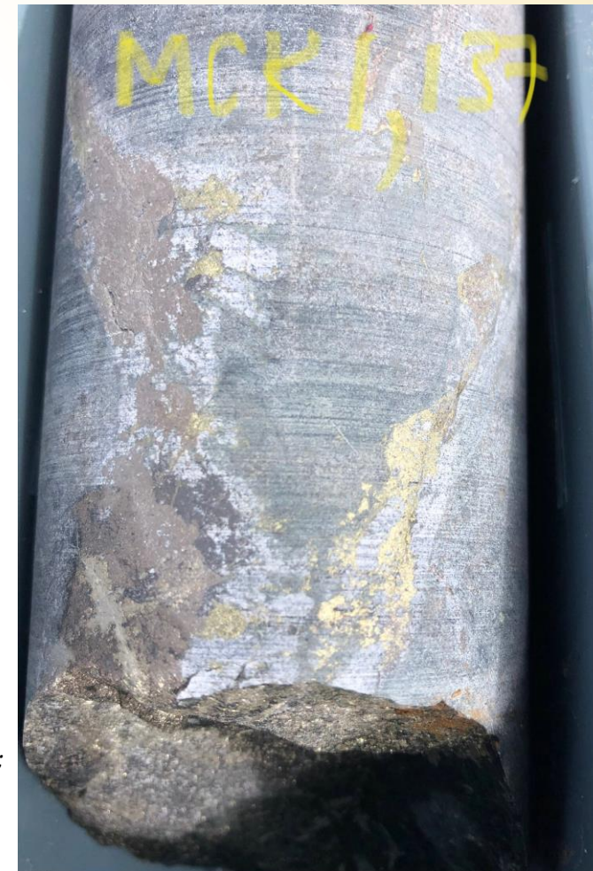
Core from the Lachlan Copper's first drill hole ("MCK1"), drilled in 2020-21 at Malachite Creek prospect on EL8758. The pictured core shows chalcopyrite (copper) mineralisation with pyrrhotite.
