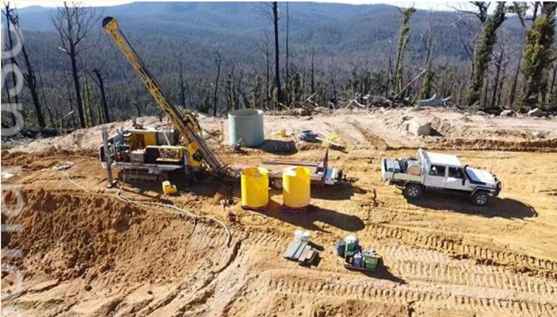
The deal includes a first right of refusal for use of this CT-14 Atlas Copco track-mounted exploration diamond drill rig, drill rods and all ancillary equipment available to County at cost.
