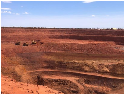
Mining Campaign 4-1 waste mining ongoing on the western cutback of the current pit
