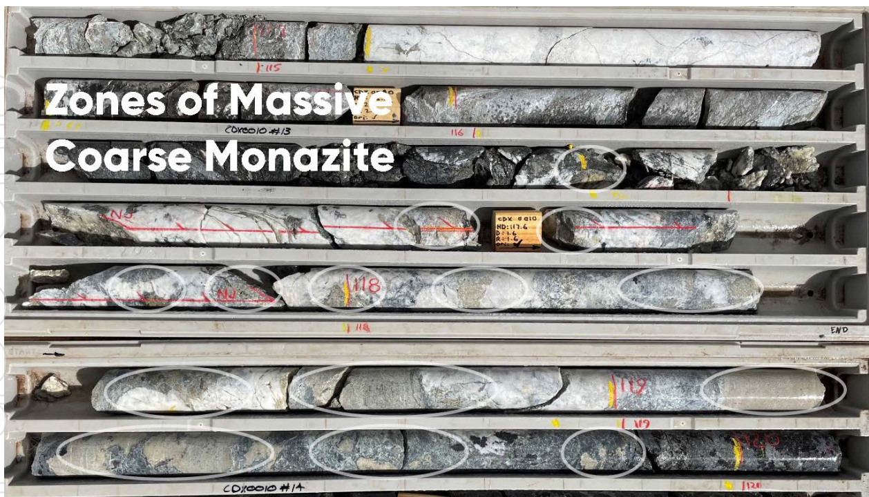
Figure 5. Patchy Massive Monazite in Hole CDX0010 – 7m at 2.3% TREO from 113m with 2m at 5.4% TREO and 0.8% NdPr.
