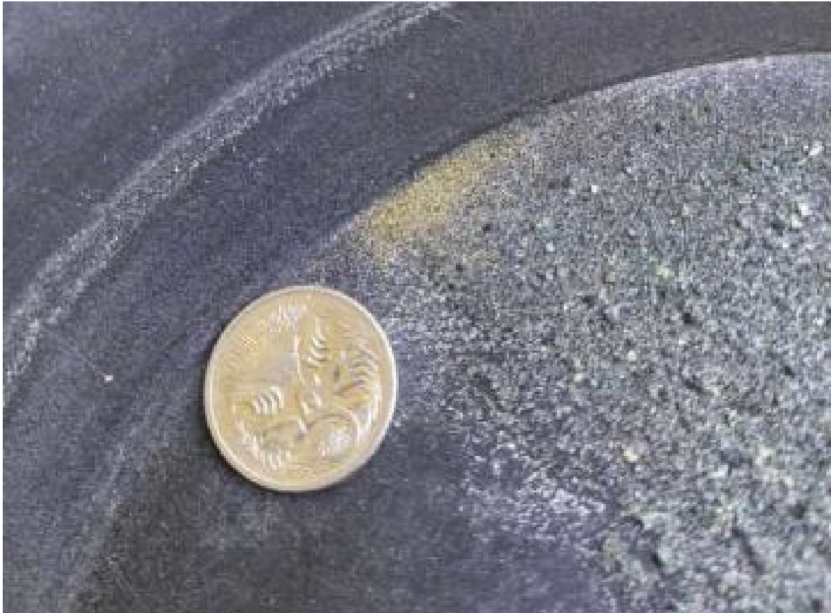
Plate 1 -Panned drill cuttings from 37- 38m MRRC01, showing gold tail
