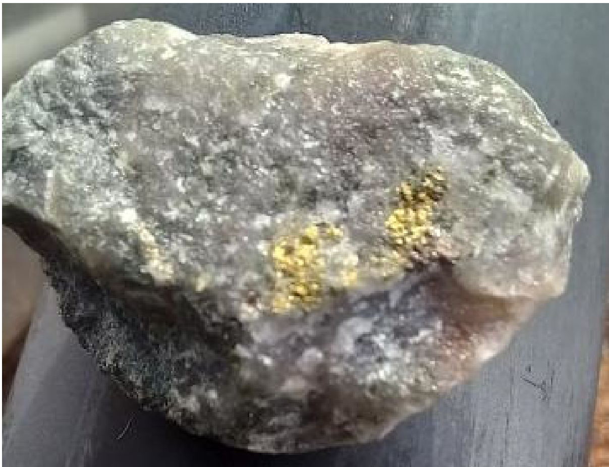
Plate 2 Drill cutting from 37-38m MRR01, showing gold/sulphides in quartz, frame view is about 15mm
