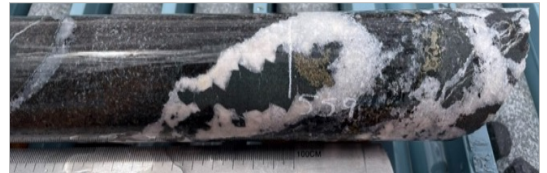
GDRCD007 - 559m, example of a quartz-calcite vein in altered diorite with pyrite \pm chalcopyrite, chlorite "Jigsaw" infill and minor brecciation.
