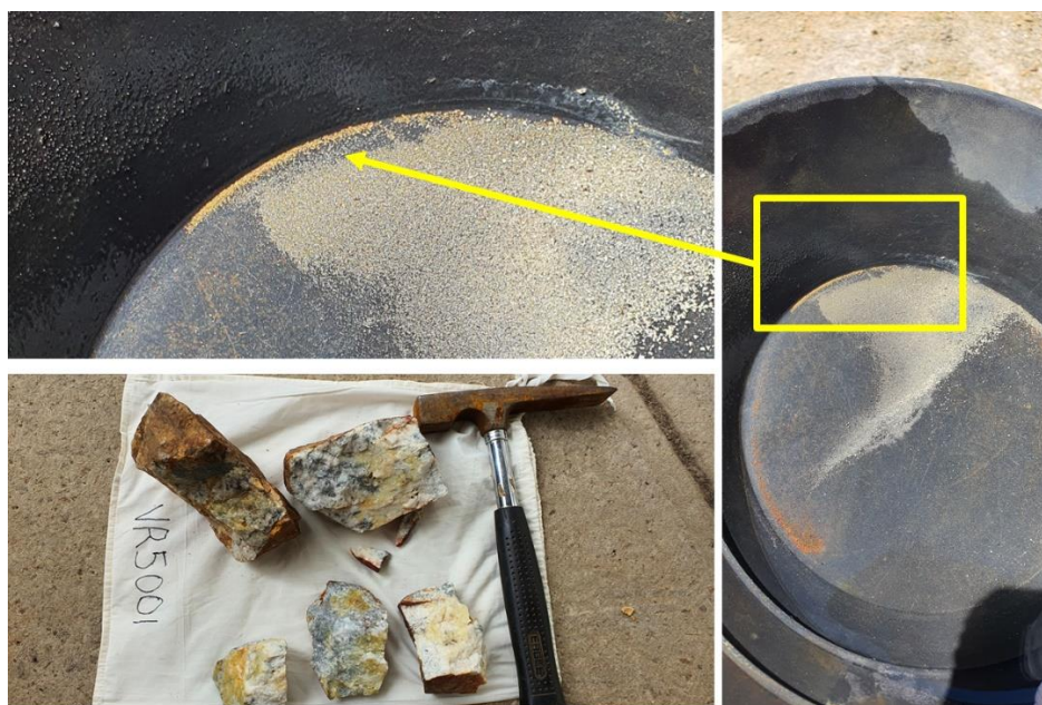
Figure 6: Reef material at surface showing evidence of free gold in the pan, resulting from trial crushing of samples collected along strike highlight the potential of the mineralised system at Snowstorm. Sample location VR5001 555805mE, 5876091mN (c.f. Figure 5 for location).
