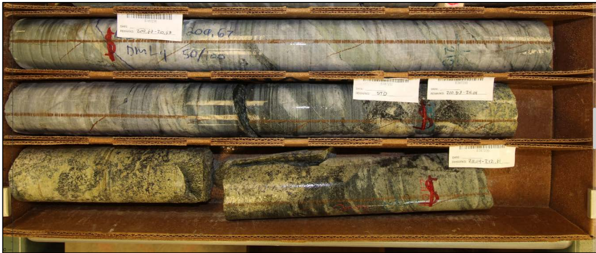
Figure 10 – Drill hole WT-21-49: core semi-massive chalcopyrite
