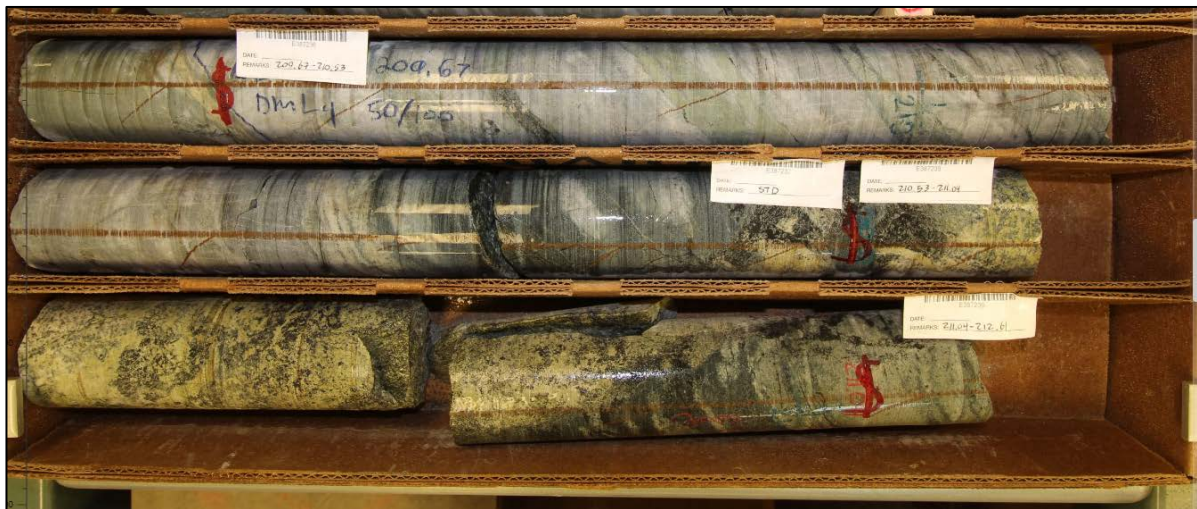
Figure 10 – Drill hole WT-21-49: core semi-massive chalcopyrite
