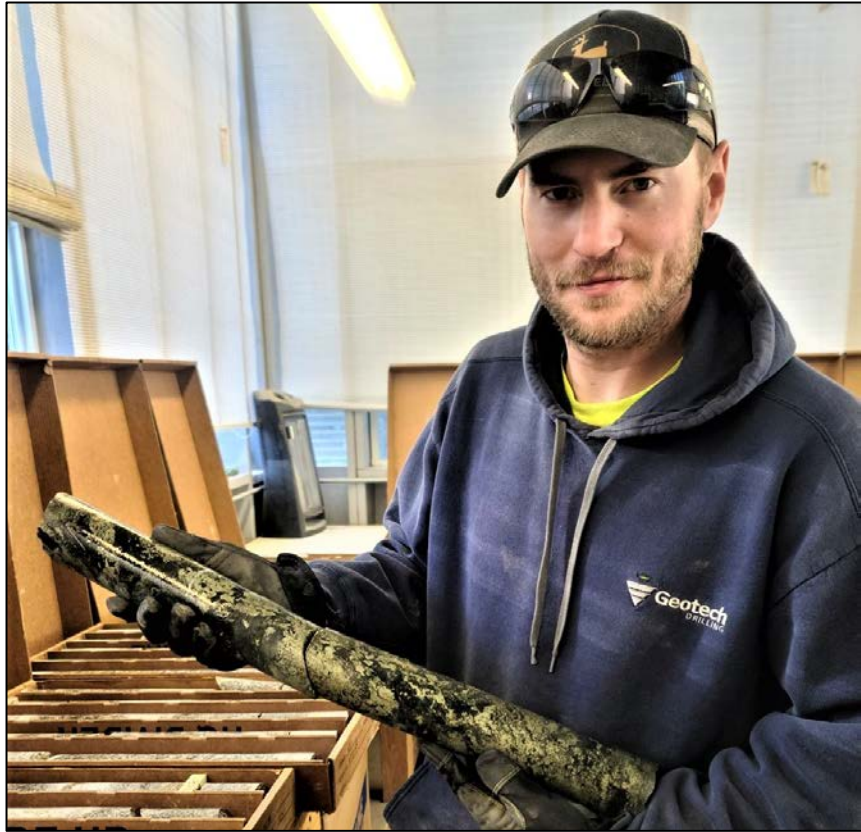
Figure 8 – Drill hole WT-21-45: semi-massive chalcopyrite (yellow copper-bearing mineral, 333.4m downhole depth)
