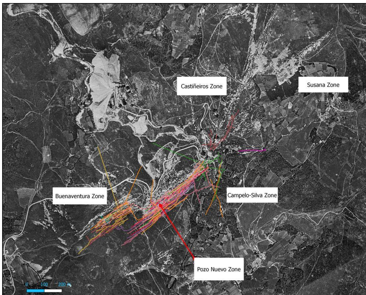
Figure 2. San Finx Sn-W deposit showing the mineralized zones at surface and the projection of the underground development for the zones of Buenaventura and Pozo Nuevo.
