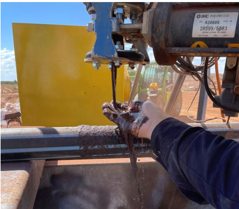
Figure 4 – First Product from Gravity Beneficiation Plant – mixed mineral concentrate
