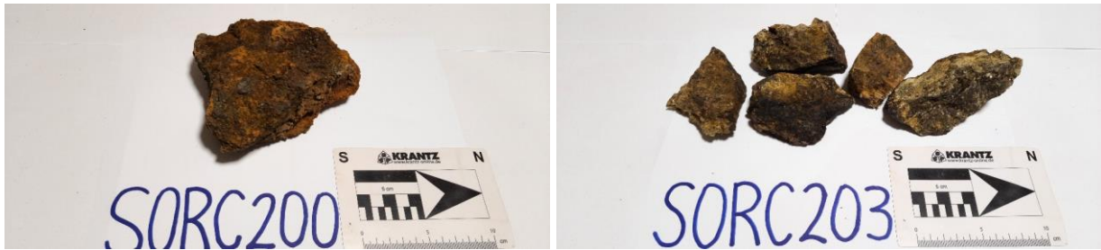
Figure 2: Samples SORC200 which returned 458ppm Co and 0.22% Ni and sample SORC203 which returned 524ppm Co and 0.45% Ni
