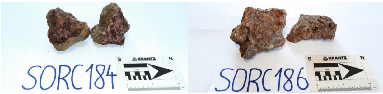
Figure 1: Samples SORC184 which returned 3.9 g/t Au, 666 g/t Ag, 6.34% Pb and 0.14% Zn and sample SORC186 which returned 5.45 g/t Au, 1,330 g/t Ag, 7.21% Pb and 5.66% Zn
