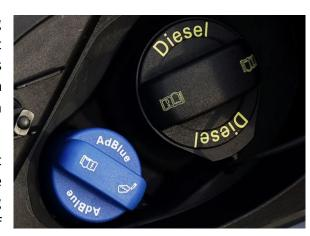
AdBlue is a non-toxic, colourless liquid. It is made from mixing demineralised (pure) water (67.5%) with high grade urea (32.5%). When injected into diesel exhaust gases, it breaks down the nitrogen oxide into nitrogen and water vapour, making the exhaust gases less pollutive and acceptable in terms of emissions standards.
