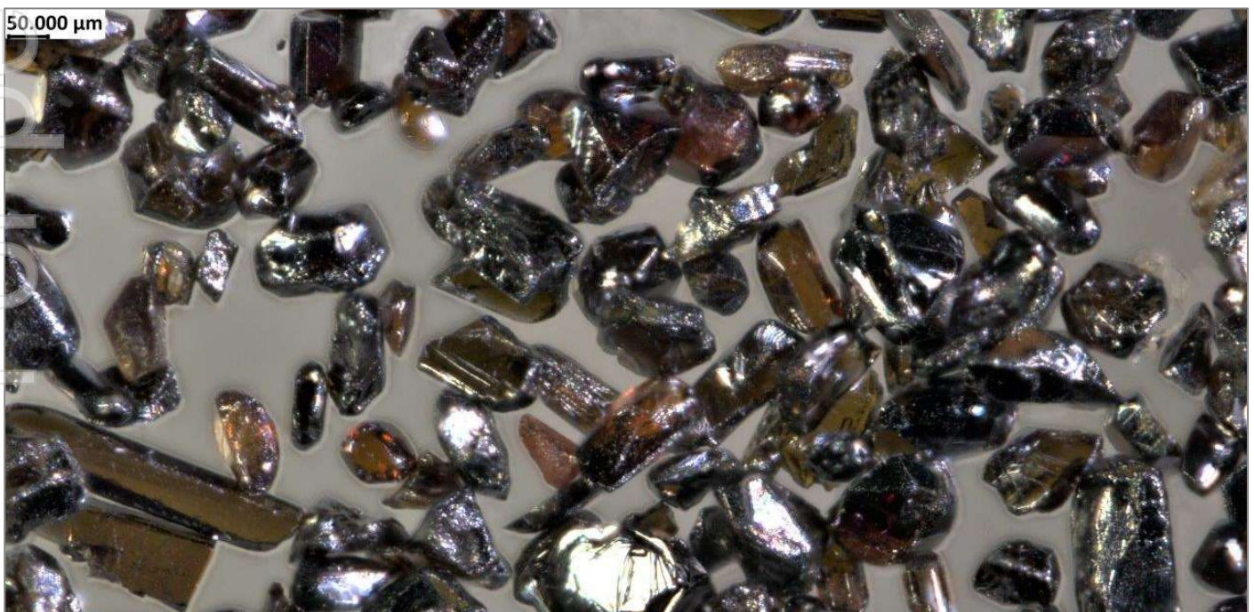
Figure 22: Photomicrograph of high purity rutile product 97.2% TiO 2
