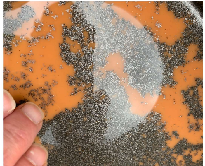
Figures 24 & 25: Very coarse-flake graphite in +600 \mu m sample fraction (L), graphite floating on soaking drill sample (R)
