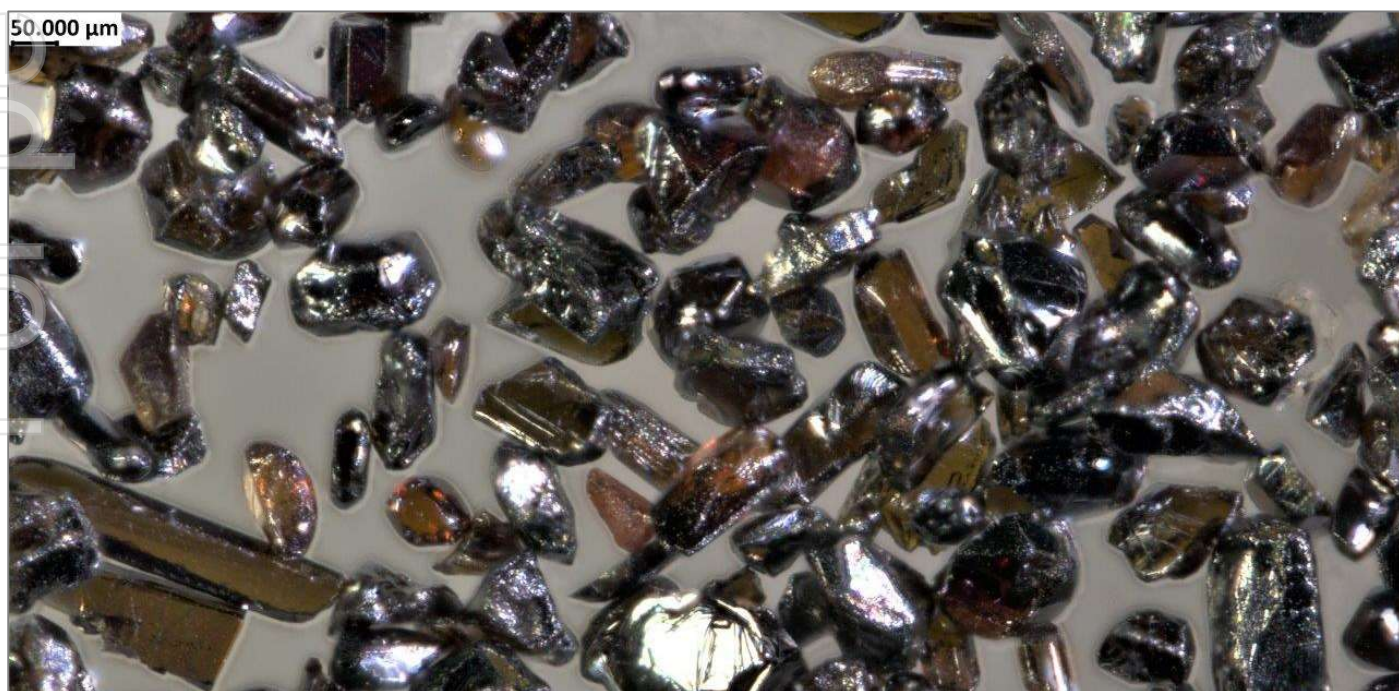
Figure 22: Photomicrograph of high purity rutile product 97.2% \text{TiO}_2
