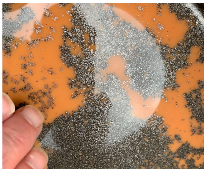
Figures 24 & 25: Very coarse-flake graphite in +600µm sample fraction (L), graphite floating on soaking drill sample (R)
