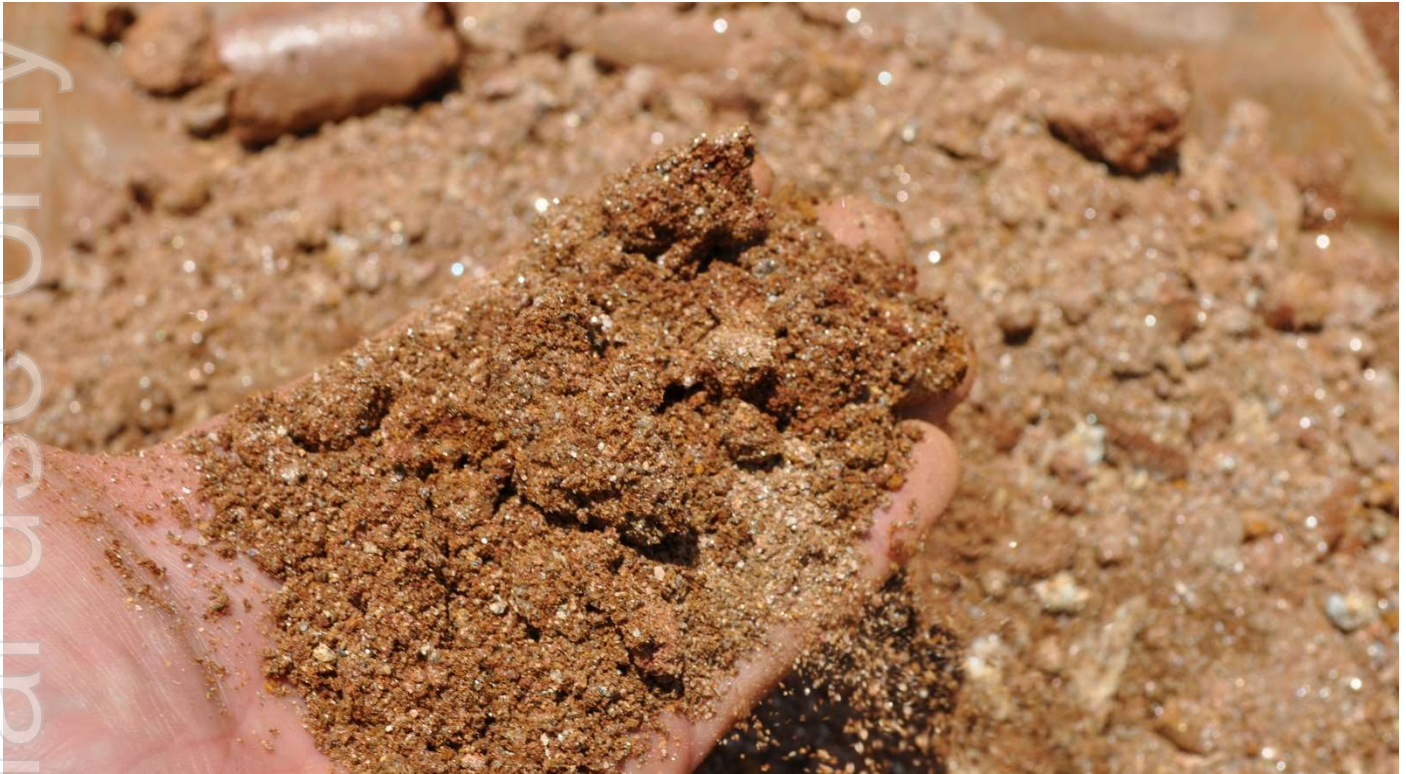
Figure 17: Kasiya saprolite hosted rutile and graphite mineralisation
