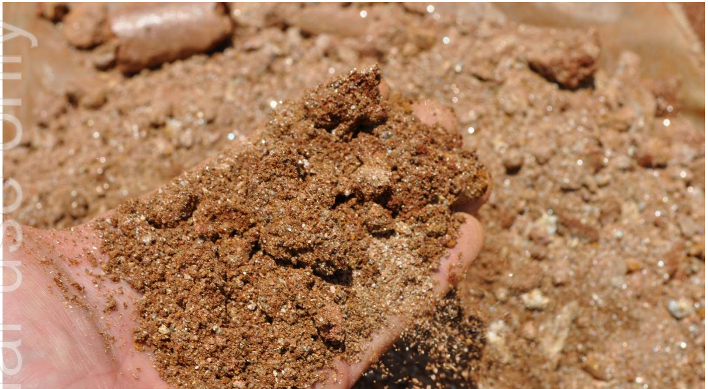
Figure 17: Kasiya saprolite hosted rutile and graphite mineralisation
