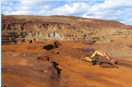
Laterite ore (1.6% nickel, 0.18% cobalt)
