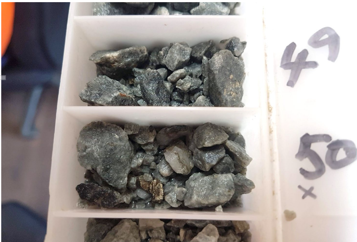
Figure 4: RC21MR002 RC chips between 49-50m highlighting pyrite-quartz veining within an interval grading 3m @ 2.92 g/t Au from 47m.
