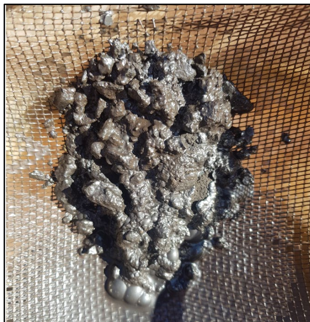
Image 10 | Sieving chalcocite rich RC drill chips 85m 21MDRC021
