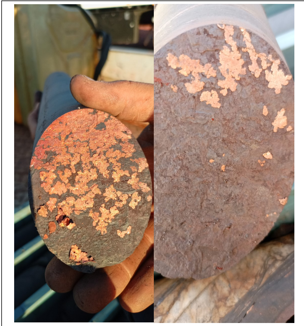
Image 6 | Native copper in carbonaceous shale 21MDMT03, 115.6m and 117.8m
