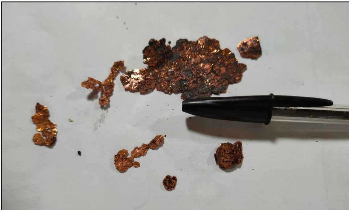
Image 4 | Native copper recovered from carbonaceous shale 21MDMT03, 114.6m
