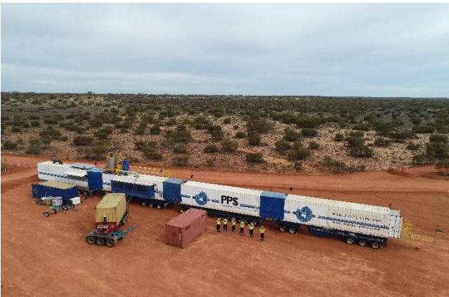
Figure 4 – PPS Extruder First HDPE pipe extruded at Ambassador (8 December 2021)
