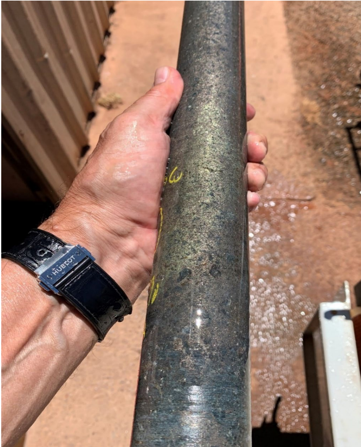
Image 1: Enriched copper sulphide interval (chalcopyrite - golden colour) hosted within 6.2m-wide zone of massive and semi-massive nickel and copper sulphides in hole ANDD0128 at VC-07 West
