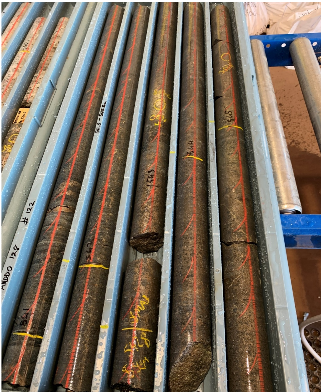
Image 2: Massive nickel-copper sulphide mineralisation in hole ANDD0128 at VC-07 West
