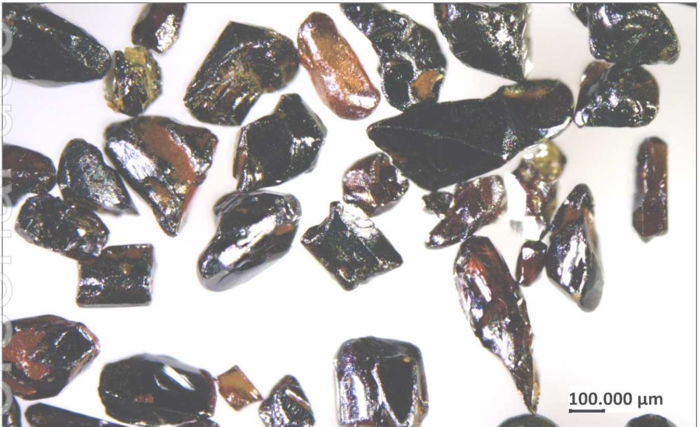
Figure 2: Photomicrograph of high purity rutile product 97.2% TiO 2
