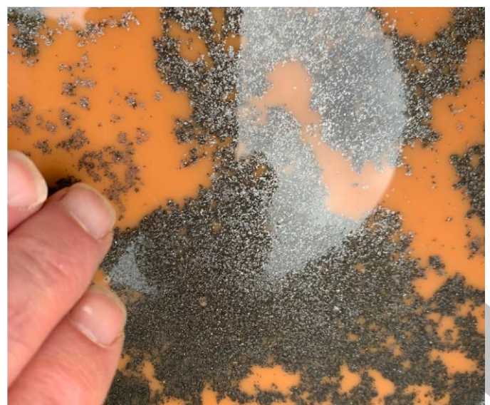
Figures 3 & 4: Very coarse-flake graphite in +600µm sample fraction (L), graphite floating on soaking drill sample (R)
