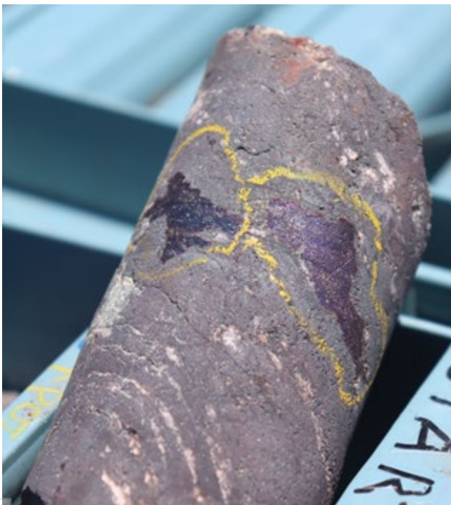
Figure 5 Mineralisation in EBD3W3B drill core. (Left) Blebby bornite with characteristic "peacock" blue/purple colouration at approx. 811m. (Below) Bedding parallel chalcopyrite mineralisation (metallic yellow mineral) associated with steely and earthy haematite (grey and red-brown, respectively) at approximately 843m.
