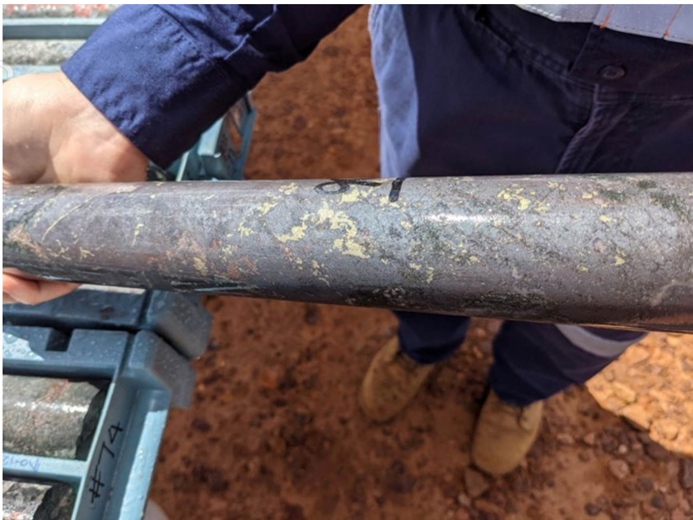
Figure 9 EBD2W3, 906m. Blebby chalcopyrite mineralisation associated with near total haematisation of sediments.
