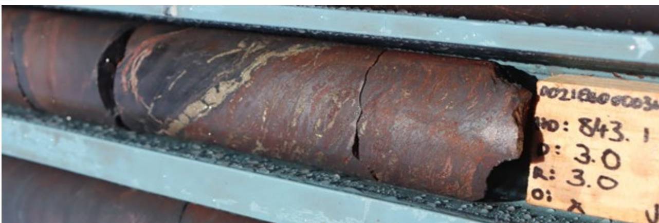
Figure 5 Mineralisation in EBD3W3B drill core. (Left) Blebby bornite with characteristic "peacock" blue/purple colouration at approx. 811m. (Below) Bedding parallel chalcopyrite mineralisation (metallic yellow mineral) associated with steely and earthy haematite (grey and red-brown, respectively) at approximately 843m.
