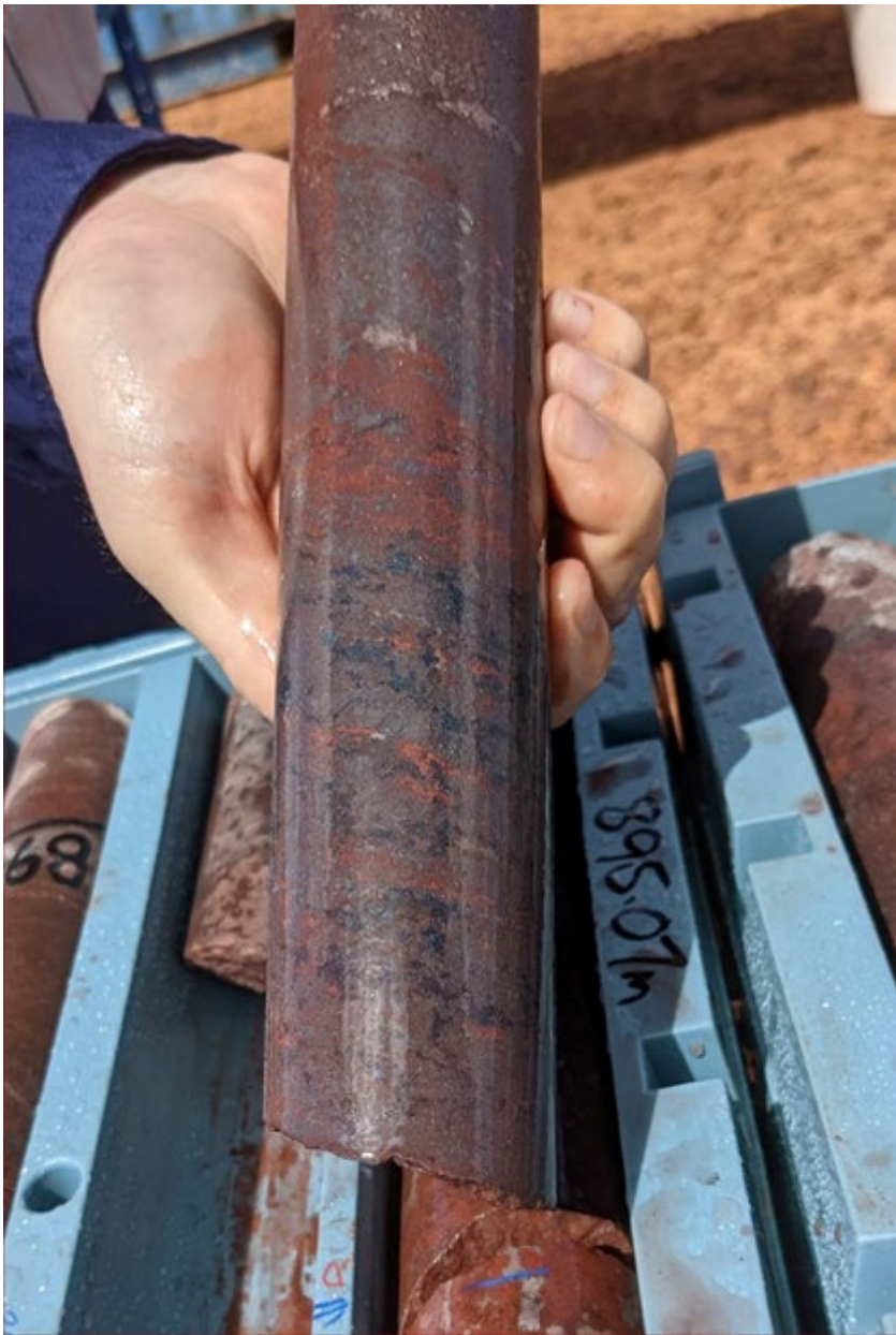
Figure 8 EBD2W3, 896m. Localised bornite mineralisation associated with a granitic intrusive.
