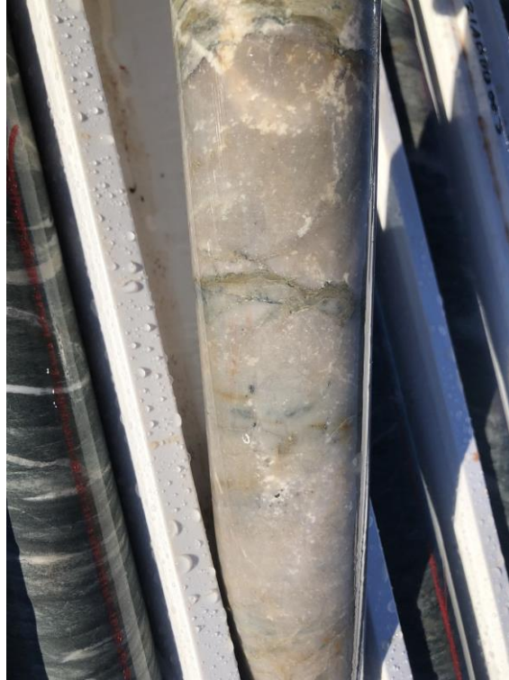
Figure 1 – 21ABDD003 (242.5-243m) showing silica flooding, carbonate altered interval with accessory pyrite, indicative of gold mineralisation.
