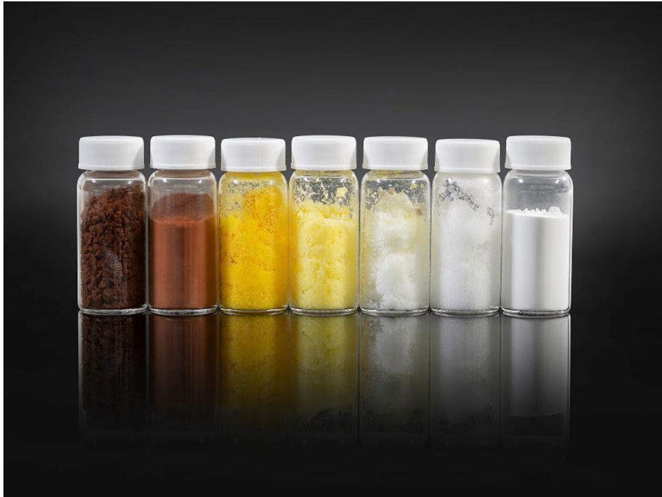
Figure: +4N HPA at right manufactured from kaolin at left with intermediary products in the vials between.
