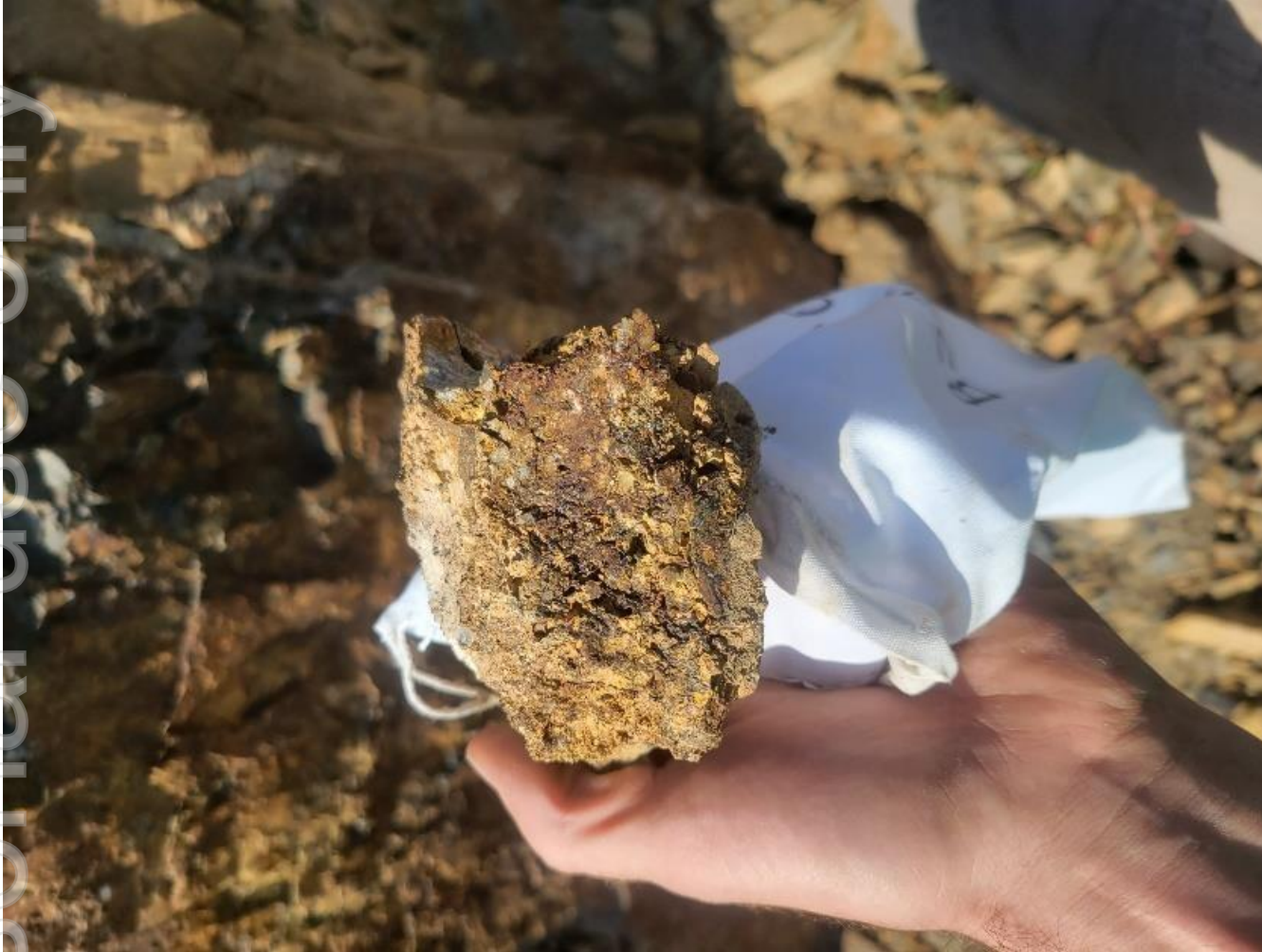
Surface Geology Mapping: Identification of strong FeOx alteration with jarosite and silicification developed along fault south of Crusher Zone
