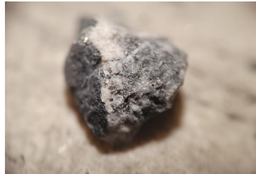
Intense sulphide alteration discovered south of Crusher Zone
