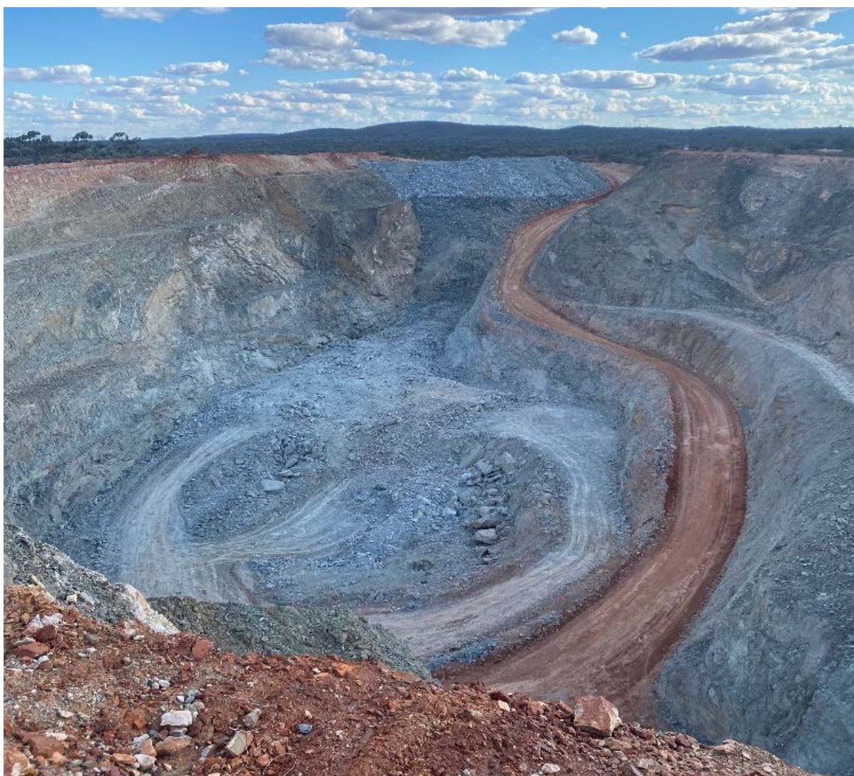
Pit Development with East-Cutback on left
