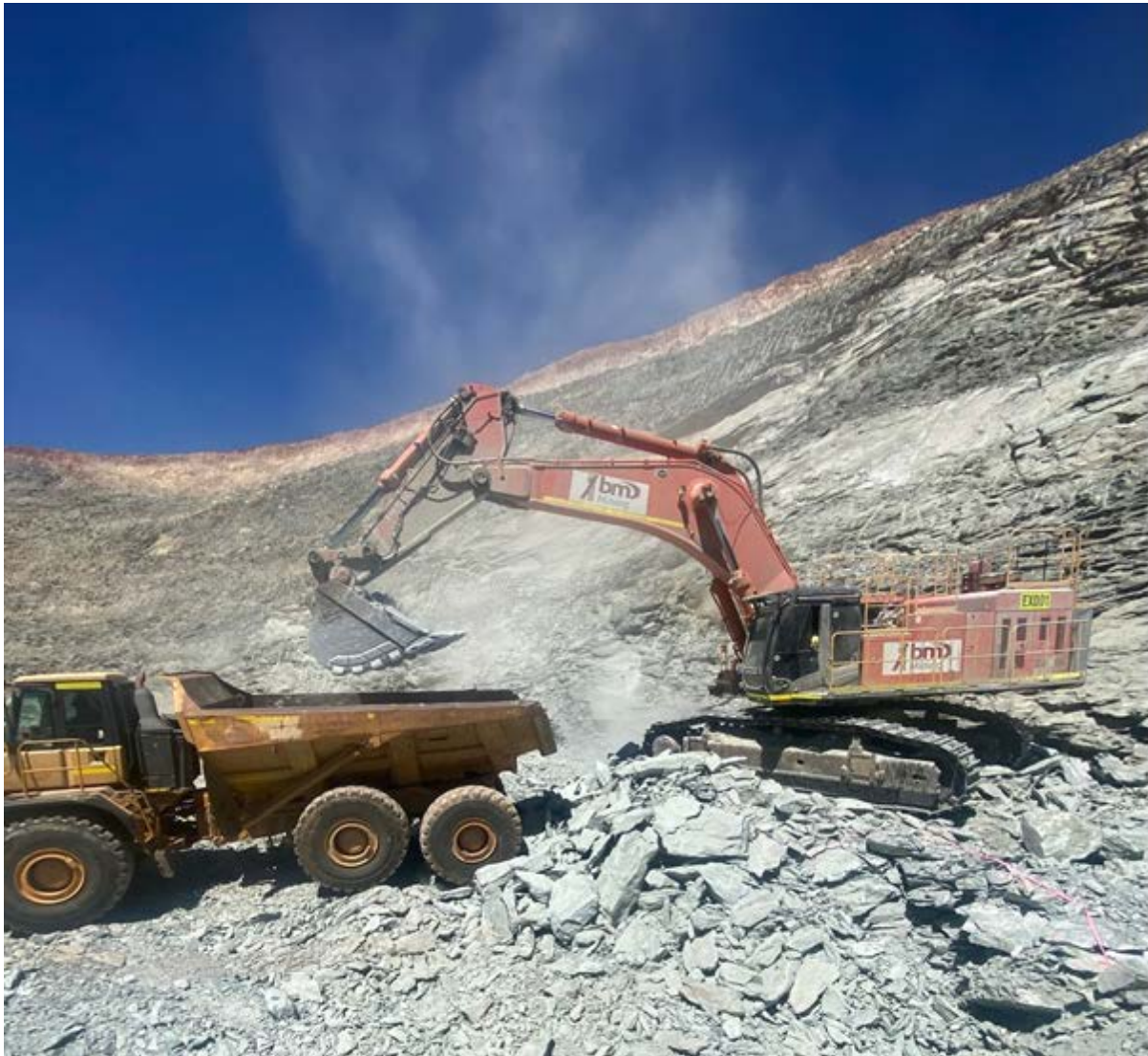
Mining ore on the top flitch of East Cut back -380mRL bench
