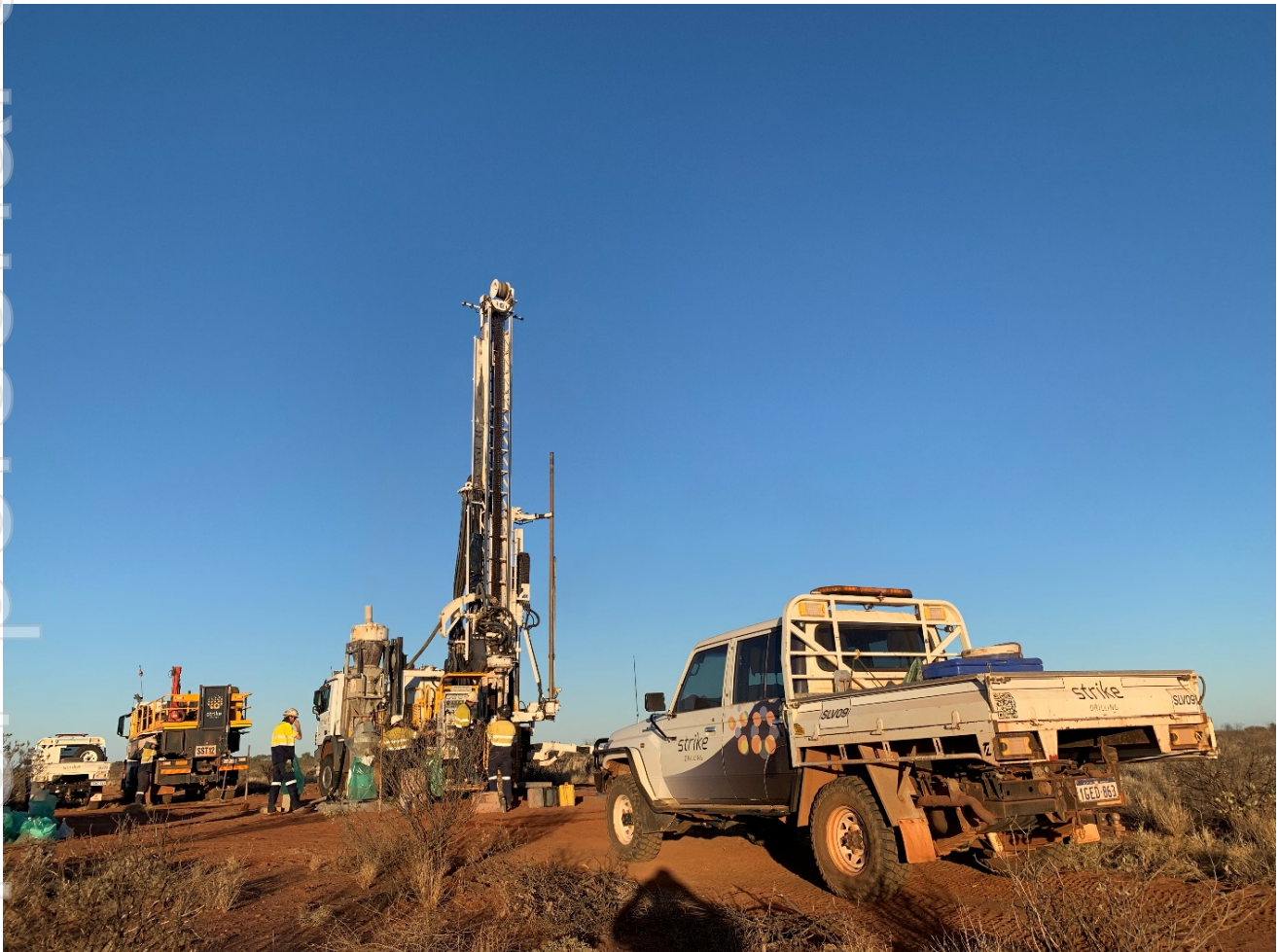
Photo 1. Strike Drilling T450 Aircore/Reverse Circulation Rig
