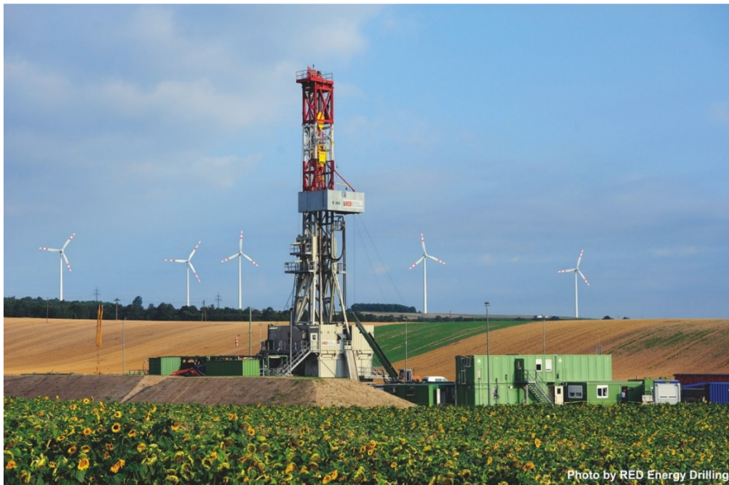
The 250 tons hook load RED Rig E-200 rig which has been contracted to drill the Anshof-3 well
