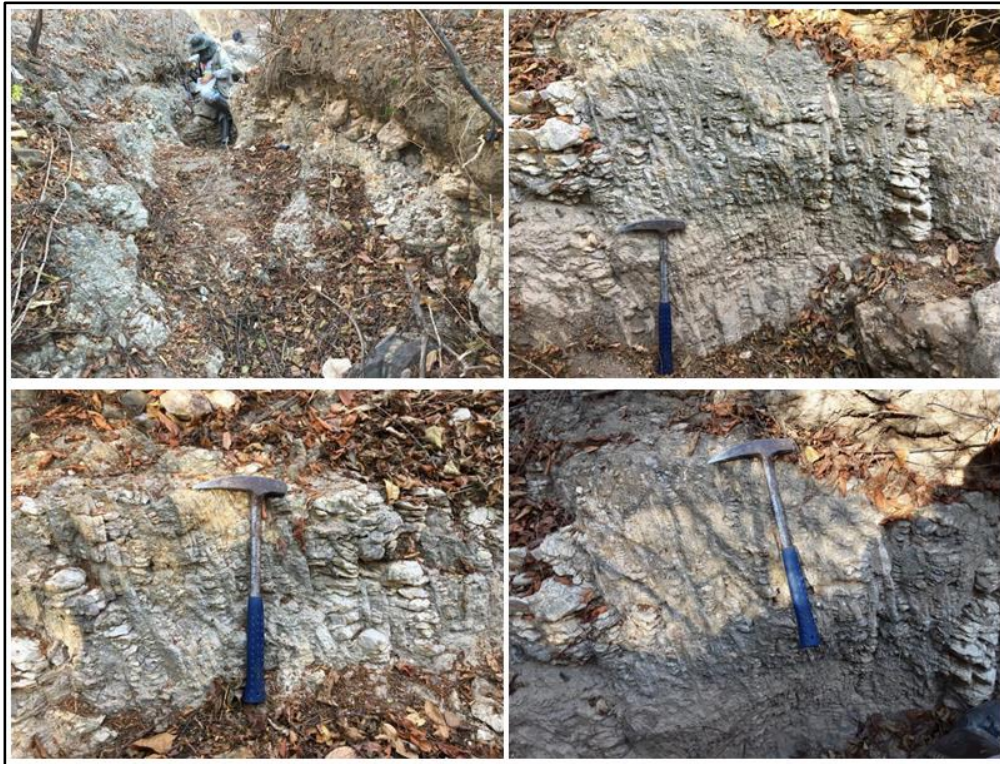
Figure 4: LRS geology team on site at the Bananal Valley Project - Mineralised pegmatite inside drainage showing highly weathered spodumene in outcrop
