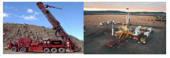
Pictured: Silver City's drill rig that will conduct monitoring, sampling of groundwater sampling wells and confirm 3D seismic survey results (left); the drill rig or similar that will be used for Stage 1 gasifiers and initiation wells (right)
