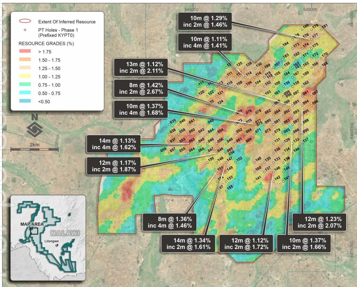
Figure 1: Kasiya core drilling plan over existing Inferred MRE block model (top block) with selected highlight hole results labelled.
