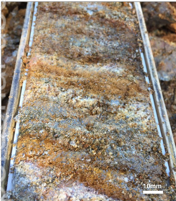
Figures 4 & 5: Coarse-flake graphite in drill core sample from Kasiya (left) & very coarse-flake graphite in the +600µm coarse sand fraction of a sized, raw drill sample (right)
