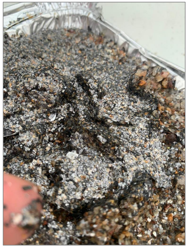
Figures 4 & 5: Coarse-flake graphite in drill core sample from Kasiya (left) & very coarse-flake graphite in the +600µm coarse sand fraction of a sized, raw drill sample (right)
