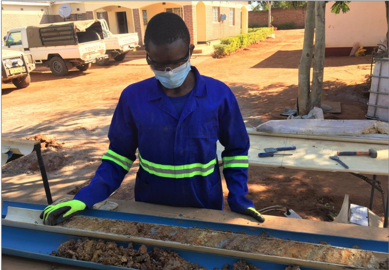
Figure 2: Sampling drill core from the push-tube program
