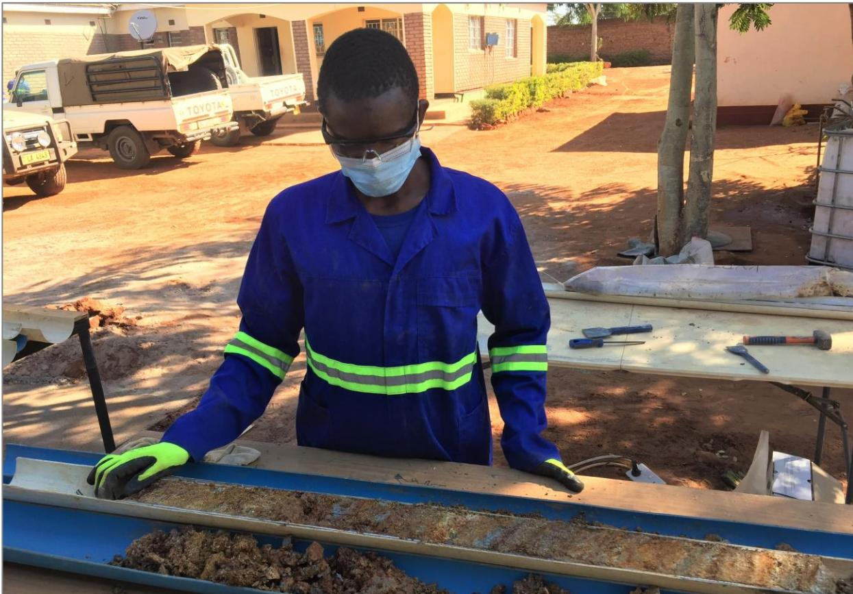
Figure 2: Sampling drill core from the push-tube program
