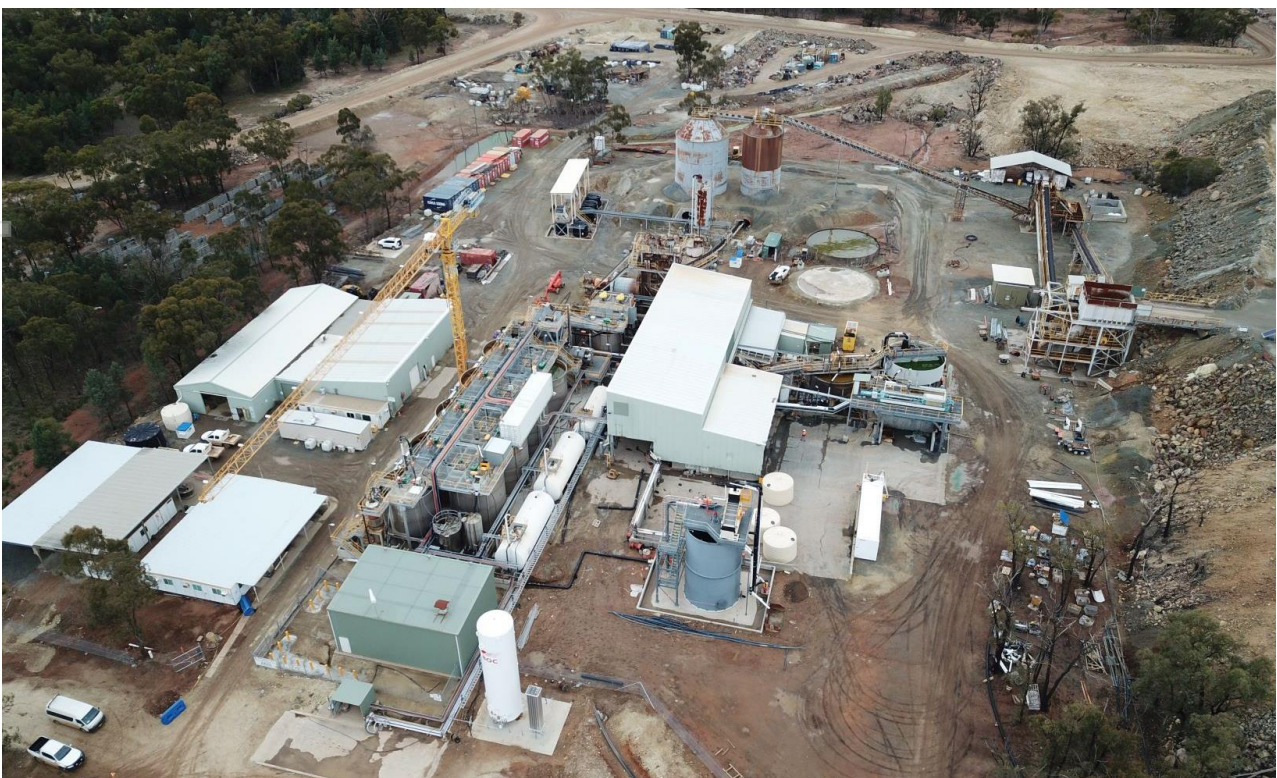
Figure 2. Site infrastructure includes a 350ktpa flotation and 400ktpa CIL circuit.
