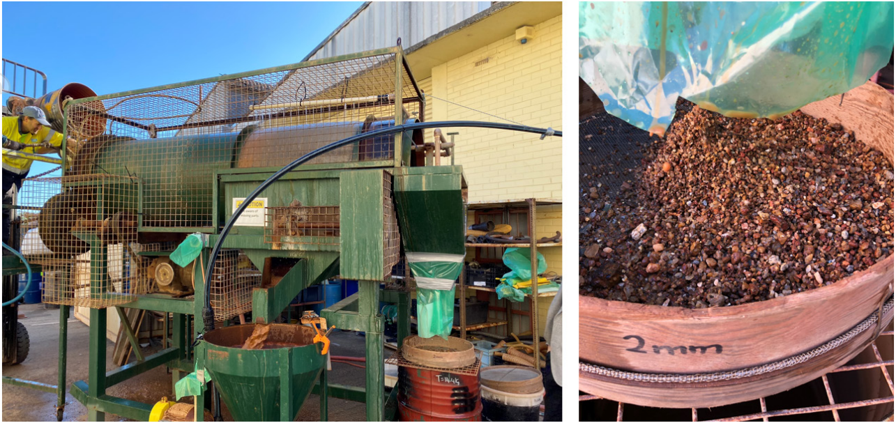
Figure 21: Trommel screen processing the raw material (left) & +2mm oversize material (right).
