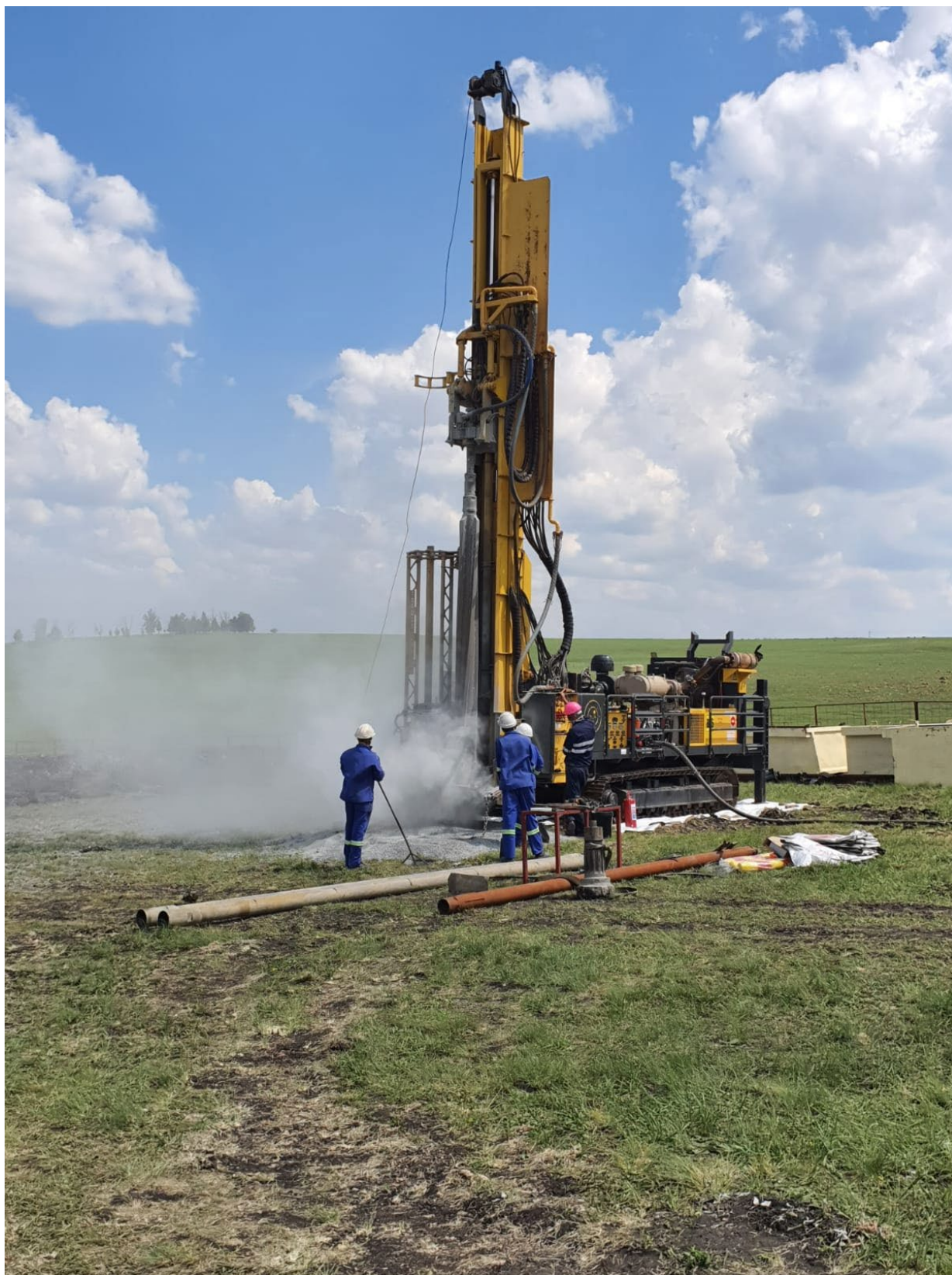
Figure 2: The B16 drilling rig spudding Korhaan-5
