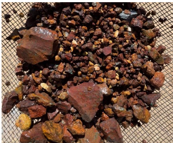
Figure 4: RC chips from KMRC047 4-5m showing oxide mineralisation comprised of gossanous iron oxides (red-brown) and secondary copper carbonates (green).
