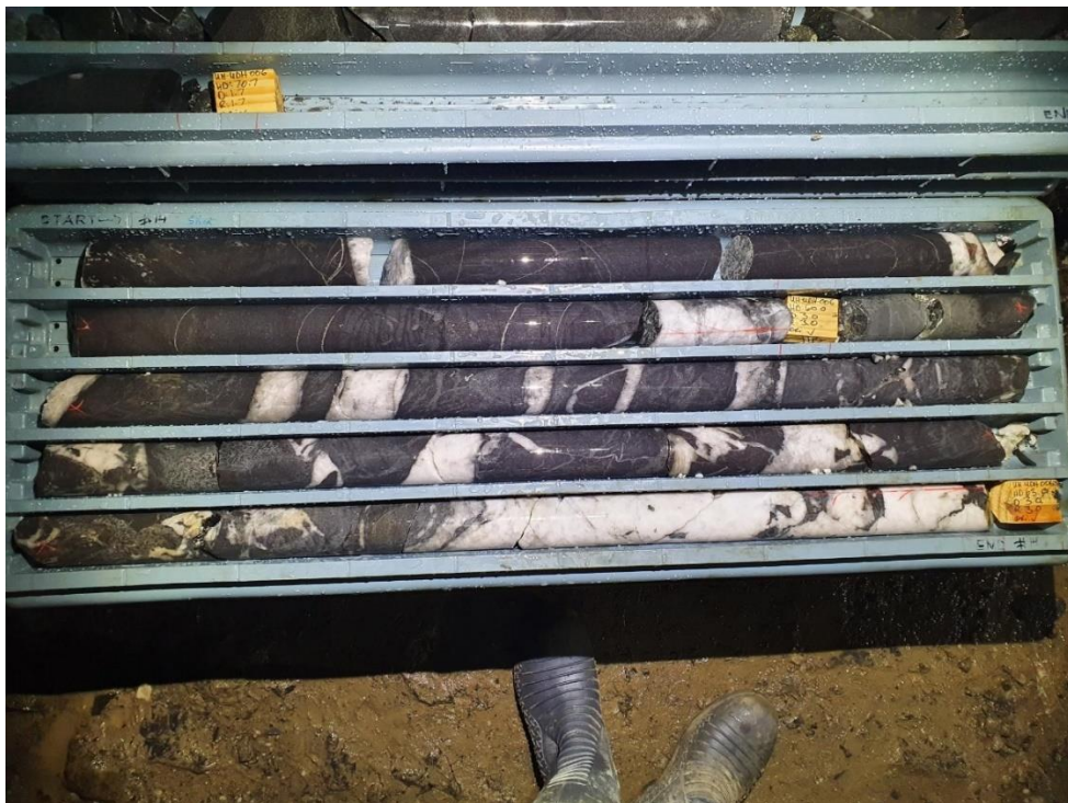
Figure 2: Eaglehawk reef showing typical mineralised quartz/sulphide lodes, UH-UDH-006: 59.73m to 61.5m for 1.77m @ 29.6 g/t gold
