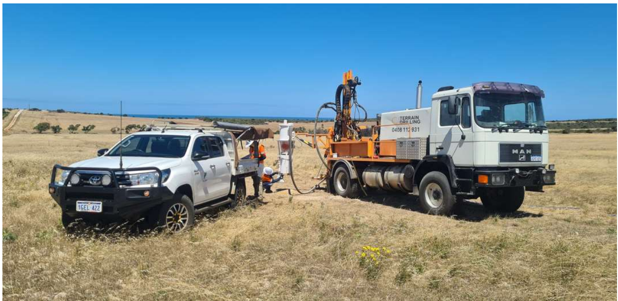
Figure 5: Terrain Drilling AC rig actively drilling on site.
