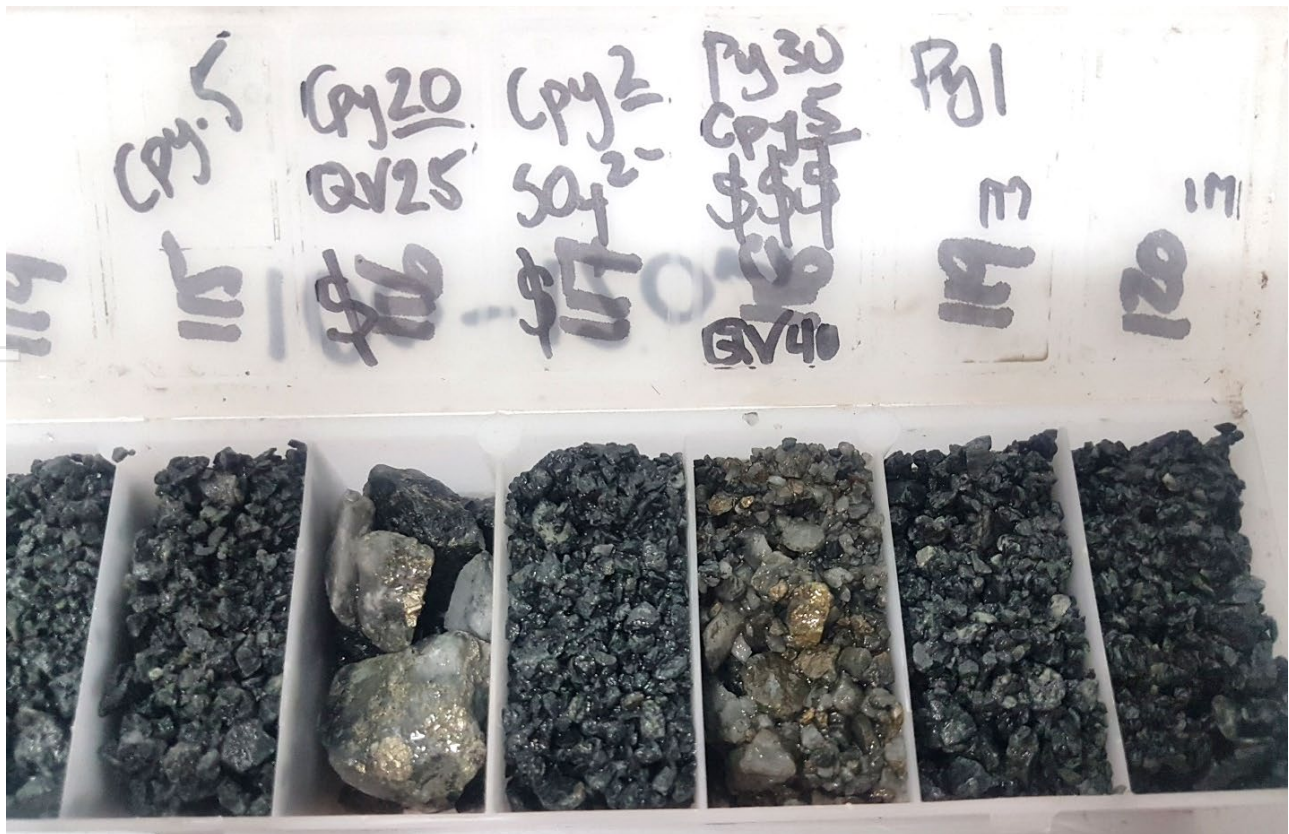
Figure 3: RC21KP1049 rock chips between 115-120m with notable 1m intersections of 4.75 g/t Au, 0.77% Cu, 5.6 g/t Ag between 115m-116m and 3.14 g/t Au, 2.59% Cu, 32.4 g/t Ag between 117m-118m.
