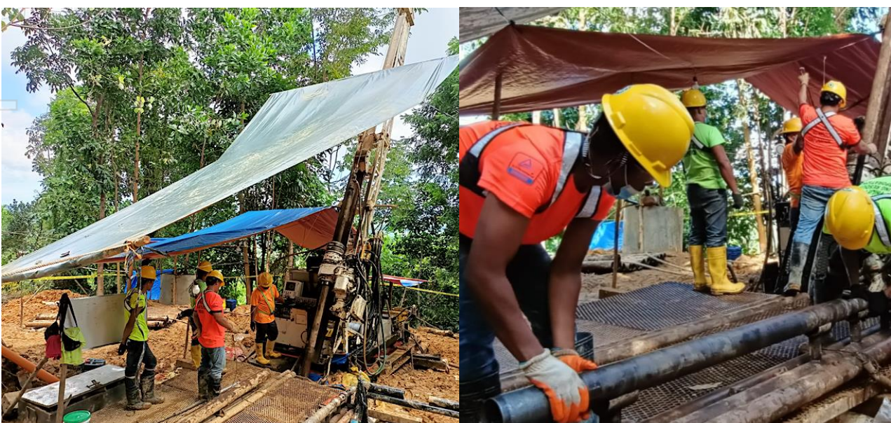
Figure 2: Drilling contractor SBF operating the diamond drill rig at the Sagay Project.
